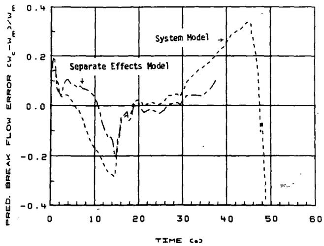
Fig. 4 Error in the RELAP4/MOD6 calculated mass flow rate for Marviken Test 11.
