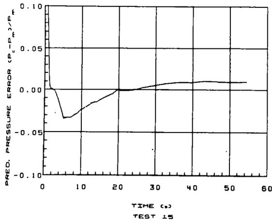
Fig. 3 Error in the RELAP4/MOD6 calculated pressure at the vessel top for Marviken Tests 6, 11, 12, 13 and 15.
