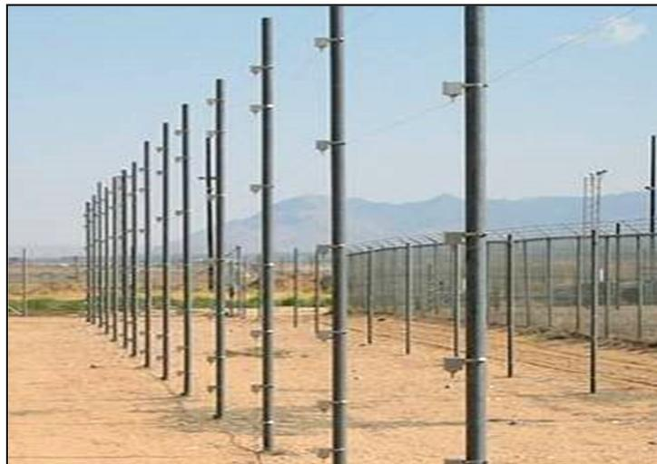
**Figure 10** Example of an electric field sensor installed in a test environment
