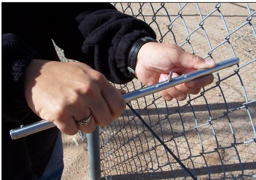
**Figure 34 Use of a fence-cut simulation tool**
