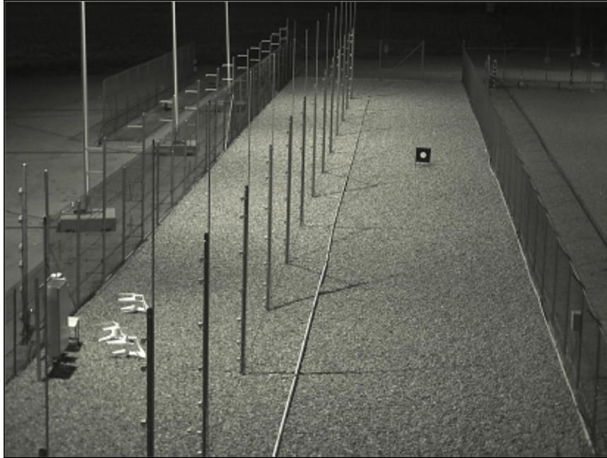
**Figure 70 Improved assessment visibility with even lighting and a regular ground surface**
