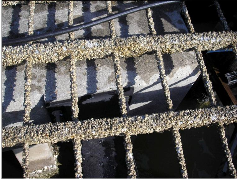
**Figure 58 Example of degradation of underwater fiber-optic grid sensors**
