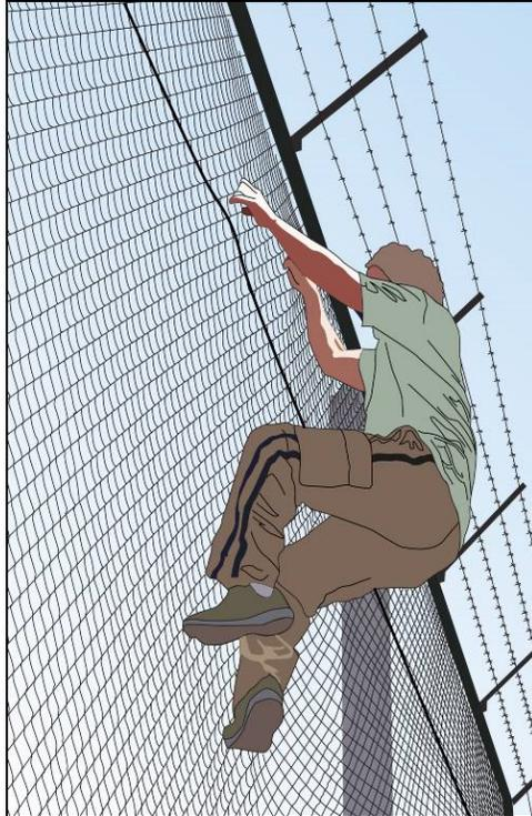
**Figure 31 Deflection caused by an intruder climbing on chain-link fence fabric**
