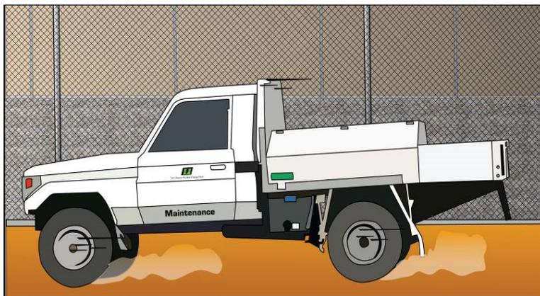
**Figure 19** Example of a nuisance alarm source for ported coaxial cable detection systems
