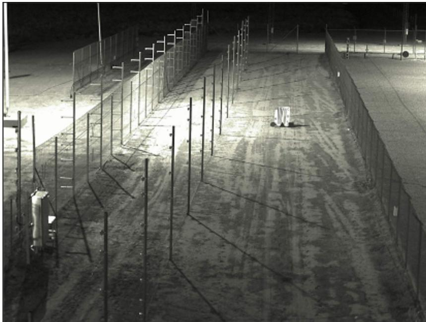
**Figure 69** Example of lighting with hot spots, dark areas, and dirt ground cover
