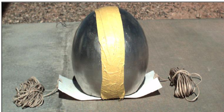
**Figure 8 Aluminum sphere used to simulate crawl tests of the microwave detection system**
