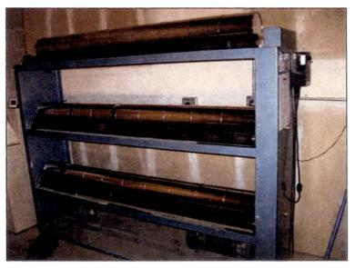
Figure 3-33 Example of Teledyne Jar Mill Machine with Sample Containers
