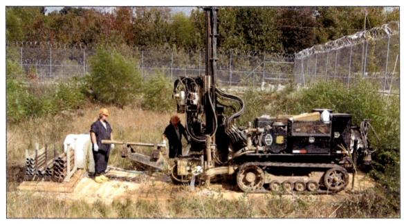
Figure 3-2 Track-mounted "Mini-Sonic" Drill Rig
