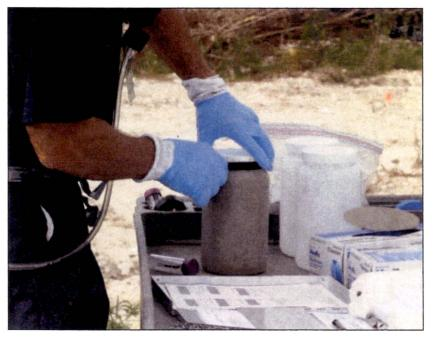
Figure 3-29 Collection of 2-L Soil Sample
