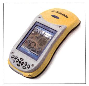
Figure 3-1 Trimble GeoXH Handheld GPS Unit
