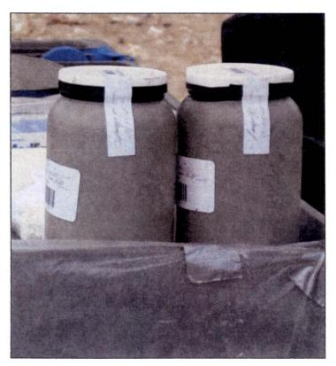
Figure 3-30 2-L Poly Jar Filled with Sample Material and Sealed
