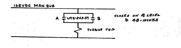
MODIFIED TURBING TRIP WITH & FEEDPUMP TRIP
