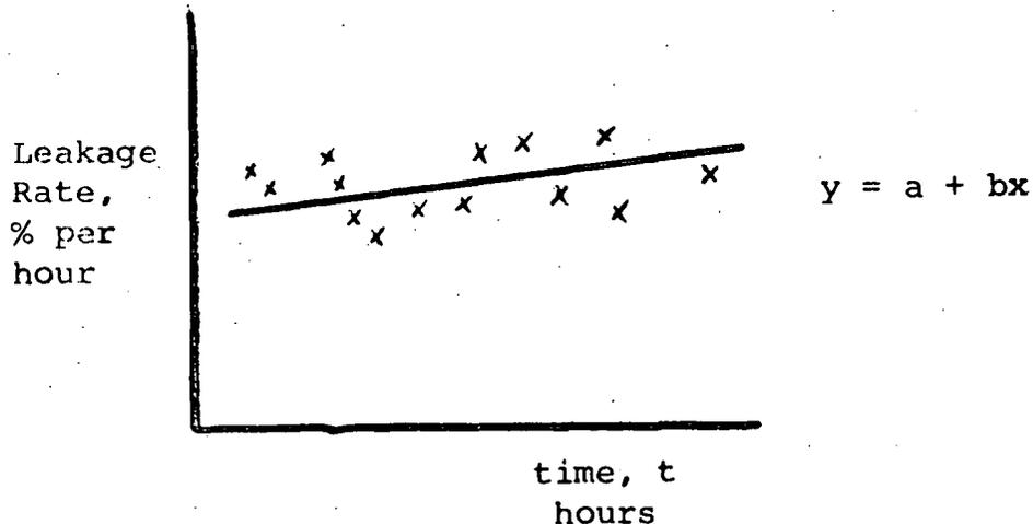
Thus the only thing accomplished is a transfer of data points to a line. We still are faced with the problem of determining an average hourly leak rate. The uncertainty calculation, on the other hand, seems quite adequate, and we feel meaningful.
