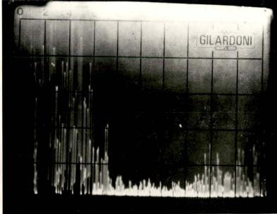
aimed at inner radius but 90° from notch. Note "clad roll" at lower right-hand quadrant. Cathode Ray Tube Portrayals of Feedwater Nozzle Inner Radius Blend
