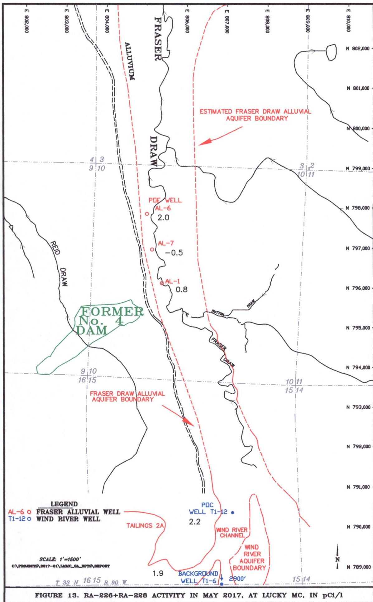
**FIGURE 13. RA-226+RA-228 ACTIVITY IN MAY 2017, AT LUCKY MC, IN pCi/l**
