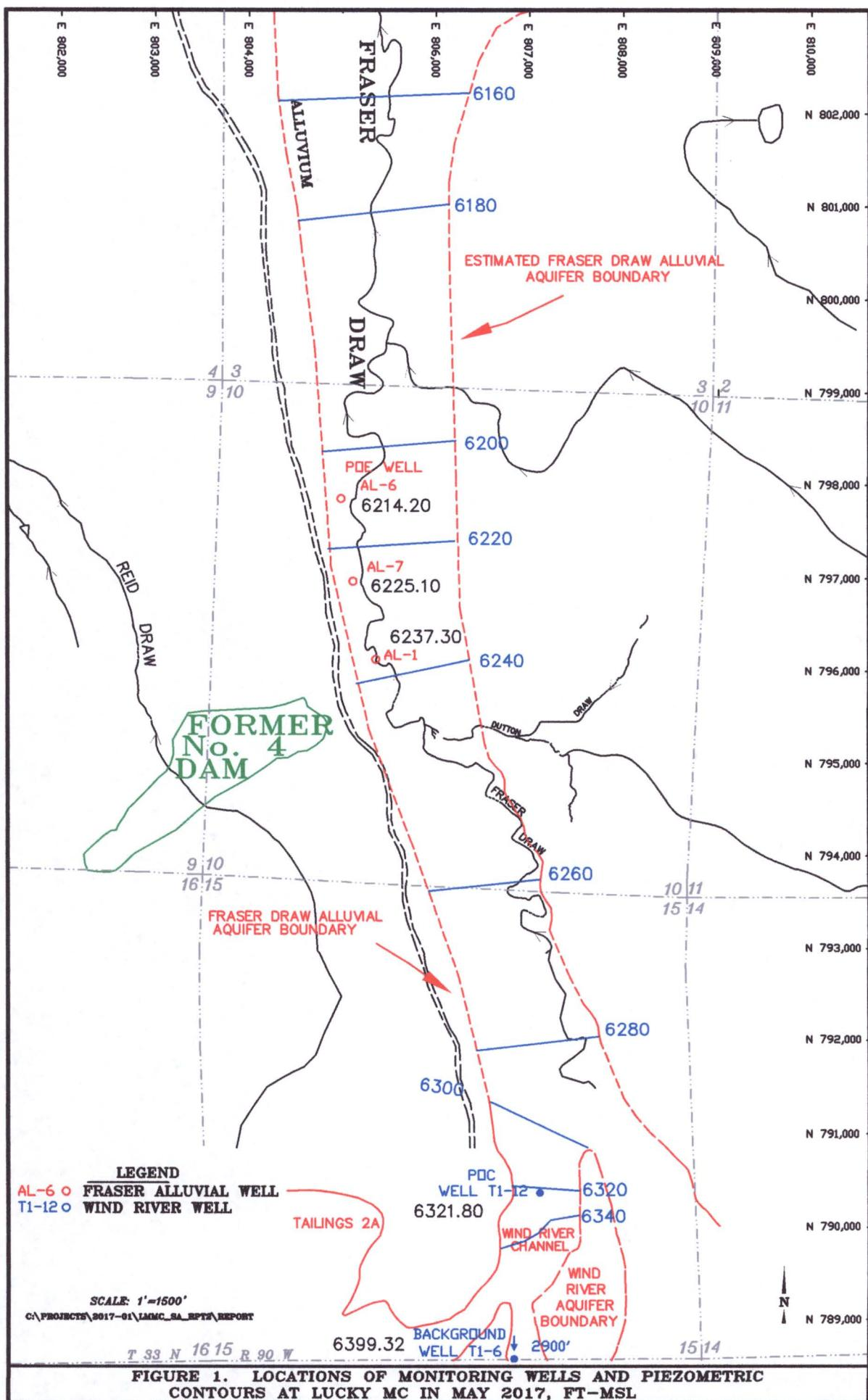
**FIGURE 1. LOCATIONS OF MONITORING WELLS AND PIEZOMETRIC CONTOURS AT LUCKY MC IN MAY 2017, FT-MSL**
