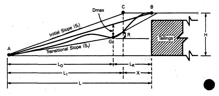
R = Angle of Repose of Cover Material
