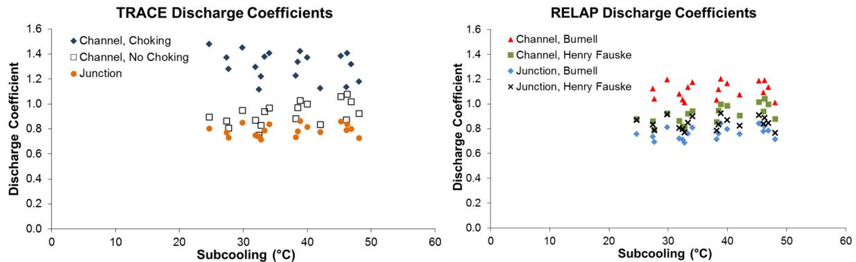
**Figure 8 TRACE and RELAP calculated discharge coefficient for Purdue tests**
