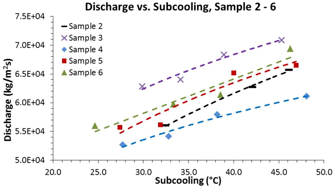
Figure 4 Critical mass flux as a function of subcooling
