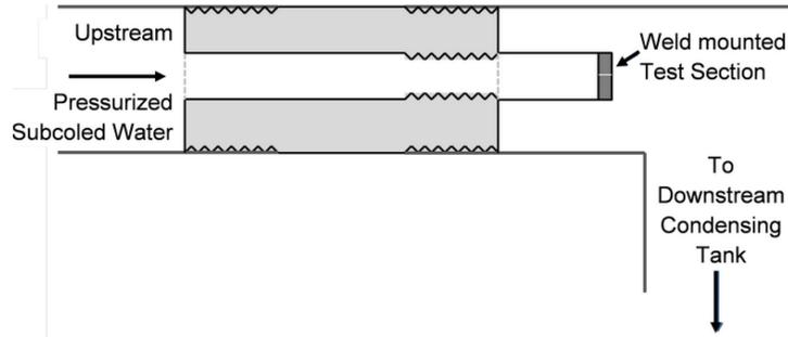
**Figure 2 Sample mounting to test section [18]**
