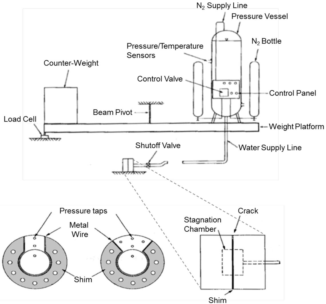
**Figure 9 Test section showing shim and the flared and rectangular crack geometries [7]**
