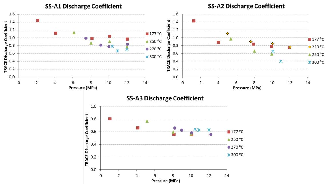
Figure 13 Discharge coefficients for the OH test samples
