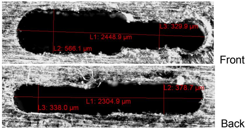
Figure 3 Slit crack test specimen # 2
