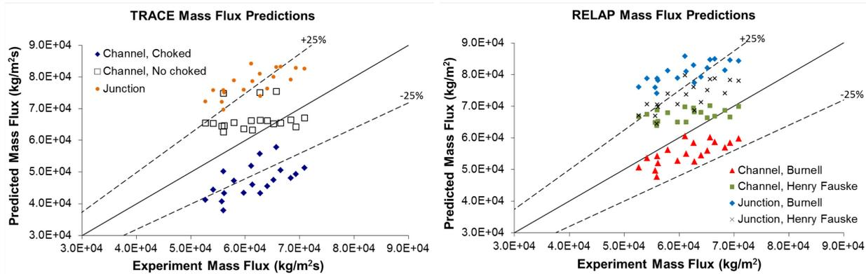
Figure 7 TRACE and RELAP mass flux predictions vs. measurements for Purdue tests
