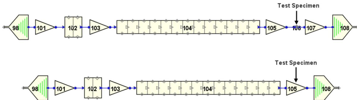
**Figure 5 RELAP channel nodalization (top) and junction nodalization (bottom)**
