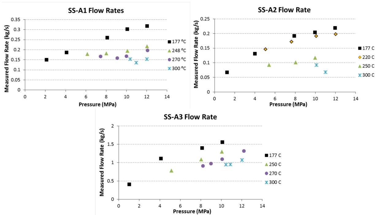
Figure 10 Measured flow rates for OH tests
