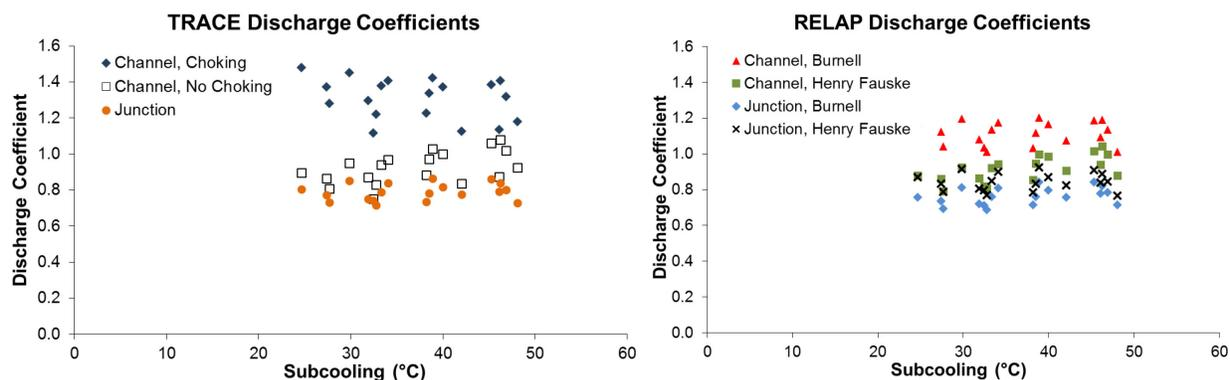
**Figure 8 TRACE and RELAP calculated discharge coefficient for Purdue tests**
