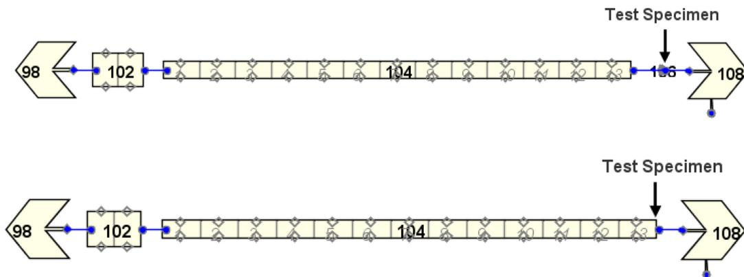
**Figure 6 TRACE channel nodalization (top) and junction nodalization (bottom)**
