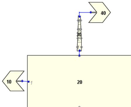
Figure 15 TRACE nodalization for the AECL tests (cell sizes not to scale)
