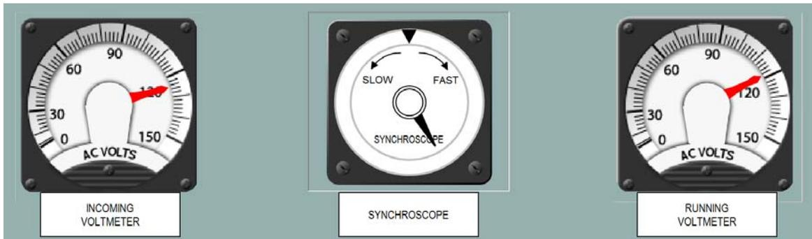
**What must the operator do to match voltage and make the Synchroscope turn 2 to 5 RPM in the FAST direction?**
