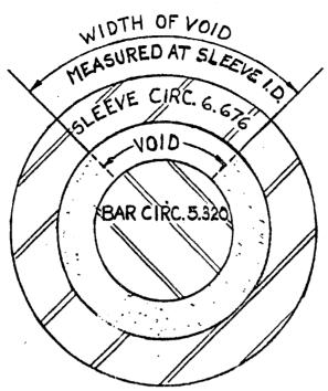
(5.320) VOID AT BAR SURFACE = .797 VOID AT SLEEVE I.D.
