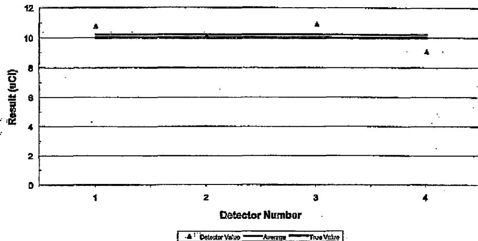
Figure 9.8: Gardian Response to a 10  $\mu\text{Ci}$  Cs-137 Button Source
