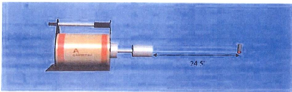
Figure 2-1: Measurement Configuration (detector aligned with point source in bottom of vial)
