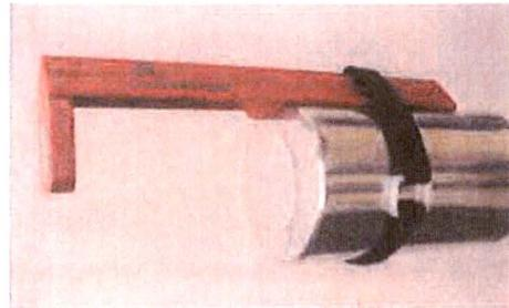
Figure 4-1: Position of Check Source and Detector for Base Line Measurements
