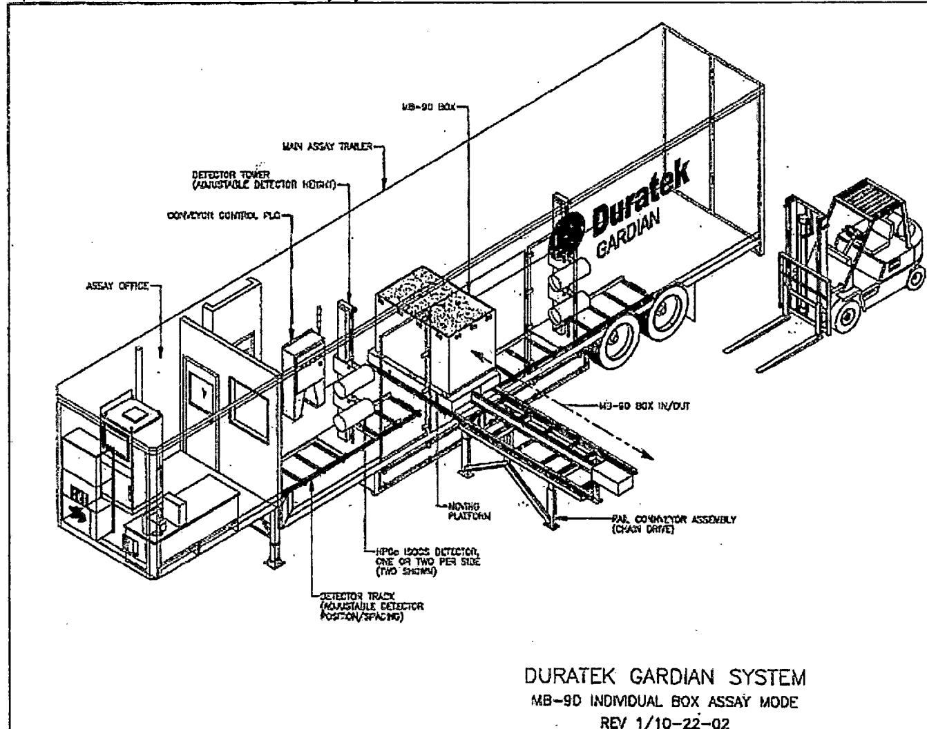
Figure 9- 3 Gardian Mobile Assay System - Box Container Mode
