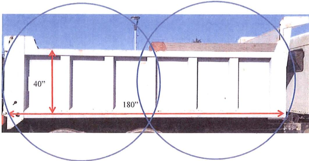
Each detector is positioned 54" from side of dump truck walls with a 90 degree collimator, giving a Field of View of 108" diameter.
