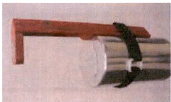
Figure 6- 1 Position of Check Source and Detector for Base Line Measurements
