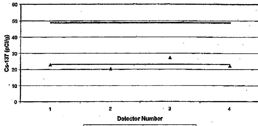
Figure 9.10: Gardian Response versus GIC Assayed Concrete Rubble
