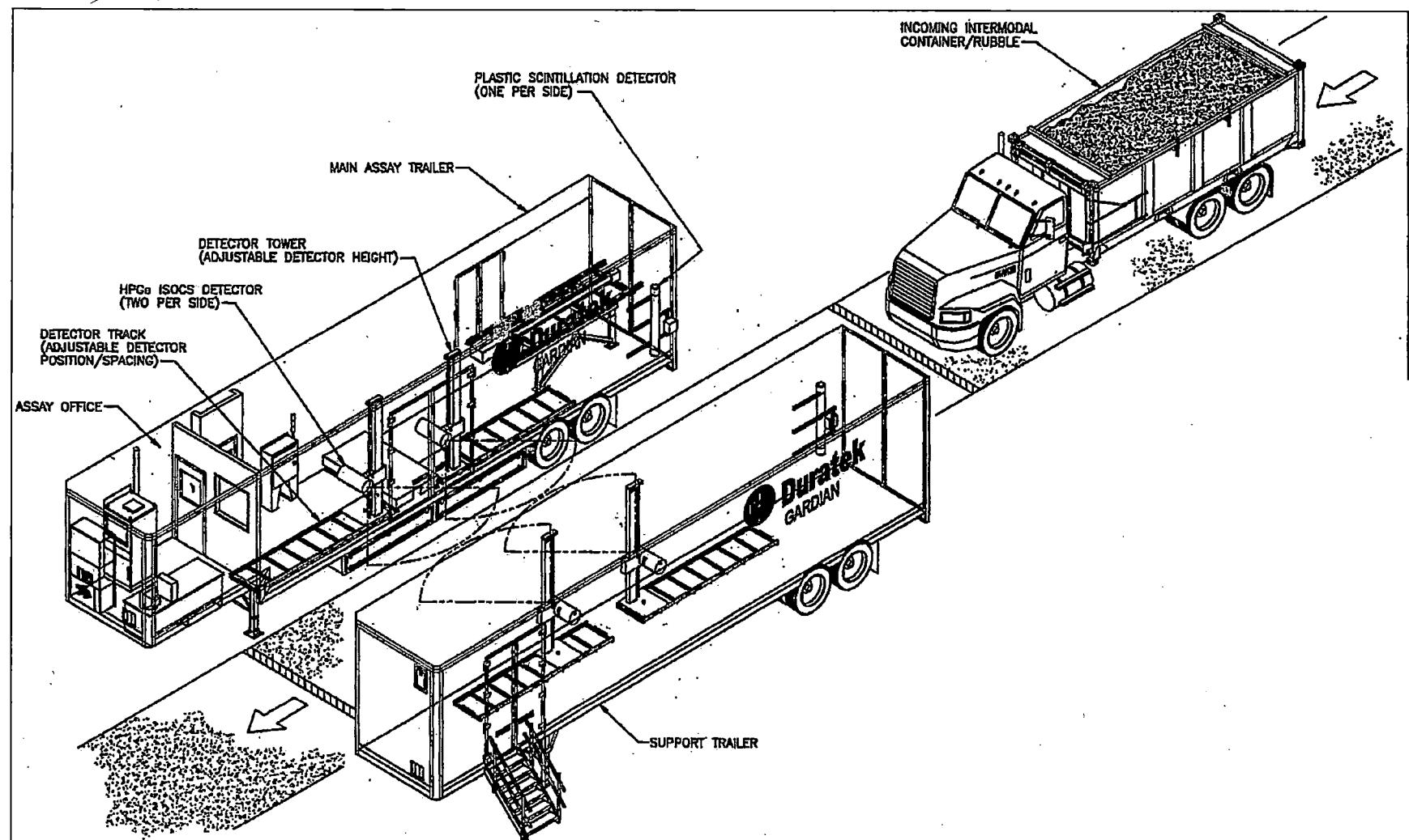
Figure 9- 1 Gardian Mobile Assay System - Large Container Mode
