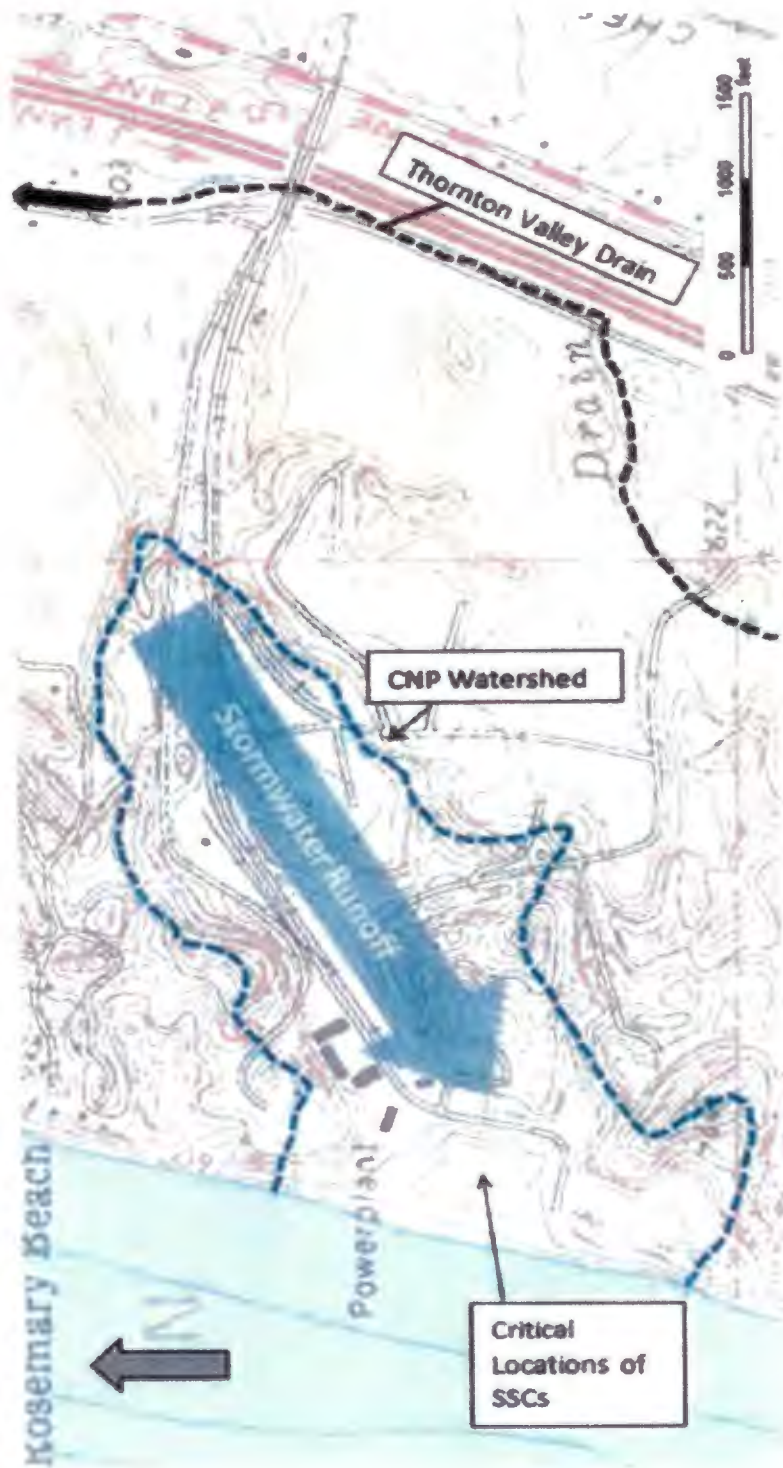
Figure 3.3-1 - Watershed draining to CNP critical locations taken from the D.C. Cook FHR Figure 3-5 (IMP, 2016a))
