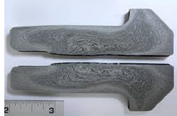
Very visible flow lines – not a BFB
