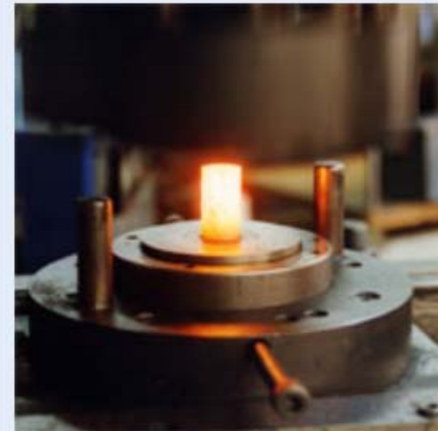
Heading press is engaged and punches down
