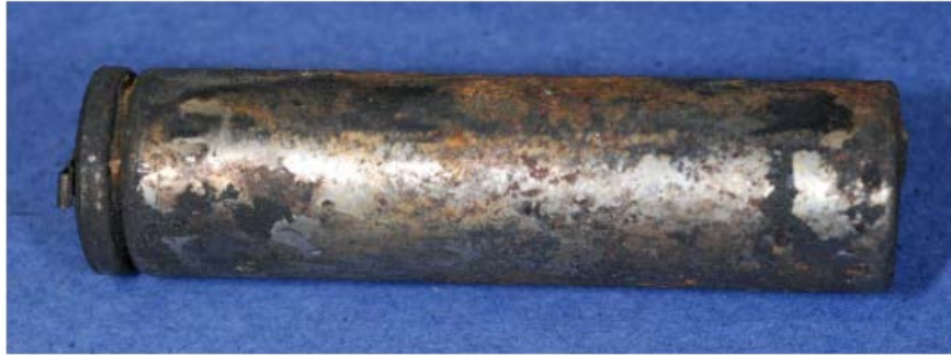
An 18650 cell that has undergone thermal runaway.
