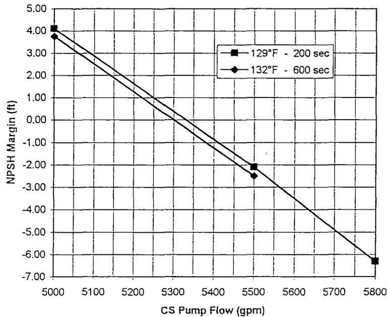
As shown above, it is expected that the Core Spray pump reduced flow due to cavitation would be greater than 5300 gpm per pump within the first 200 seconds post-LOCA. This is greater than the 5276 gpm per pump required in the first 200 seconds post-LOCA to ensure the PCT remains below 2200°F. The Core Spray pump reduced flow beyond 200 seconds would be at least 5300 gpm per pump, greater than the nominal 4500 gpm per pump that is required.
