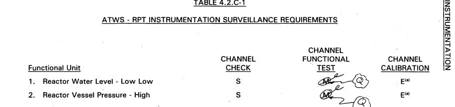
Trip units are calibrated at least once per (3) days and transmitters are calibrated а at the frequency identified in the table.
