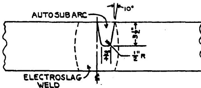
AUTOMATIC SUBMERGED ARC WELD
