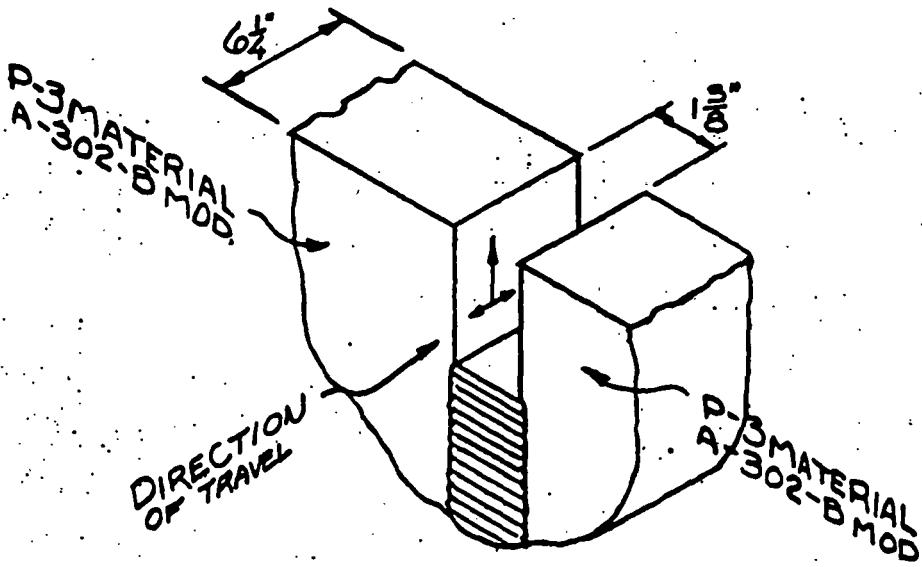
ELECTROSLAG DOUBLE ELECTRODE WELD A.C.
