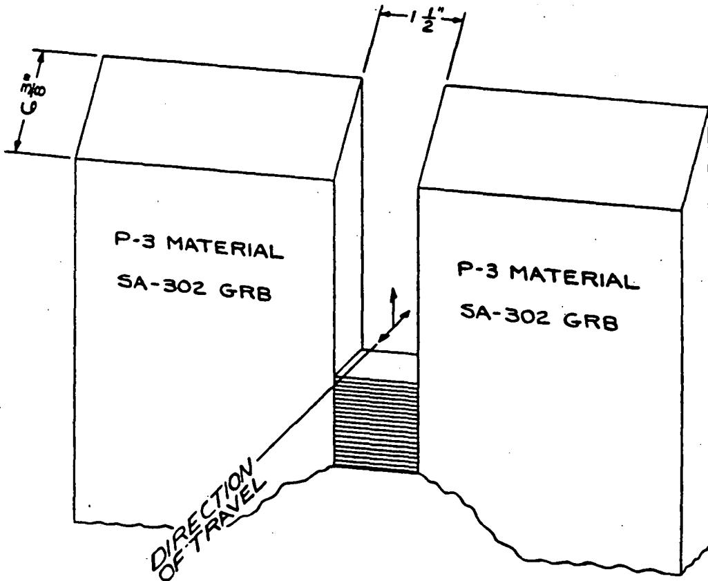
ELECTROSLAG WELD A.C. 48-52 VOLTS 575-625 AMPS
