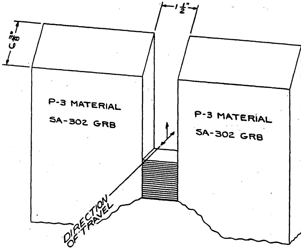
ELECTROSLAG WELD A.C. 48-52 VOLTS 575-625 AMPS
