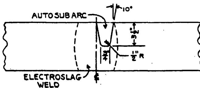
AUTOMATIC SUBMERGED ARC WELD
