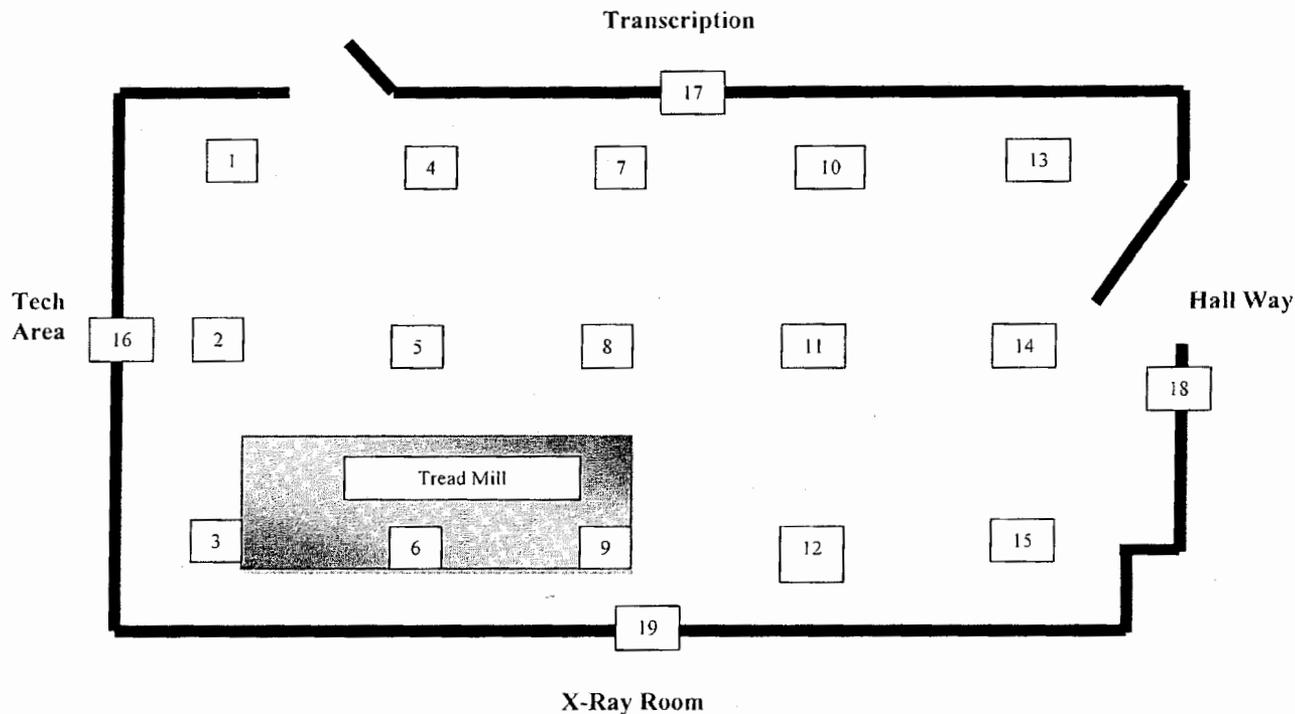
The above diagram shows the location of the wipes for detection of removable contamination during the close out survey of the Stress lab room at United Medical Center on September 14, 2014. Wipes 16, 17, 18 & 19 are gross wipes on each wall inside the room.
