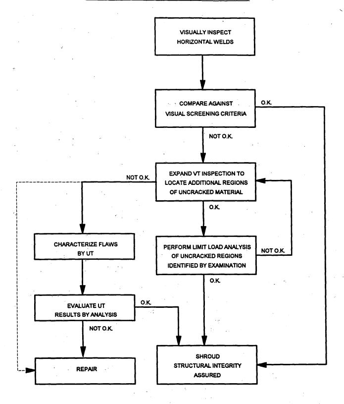
Figure 1: Shroud Inspection Flow Diagram
