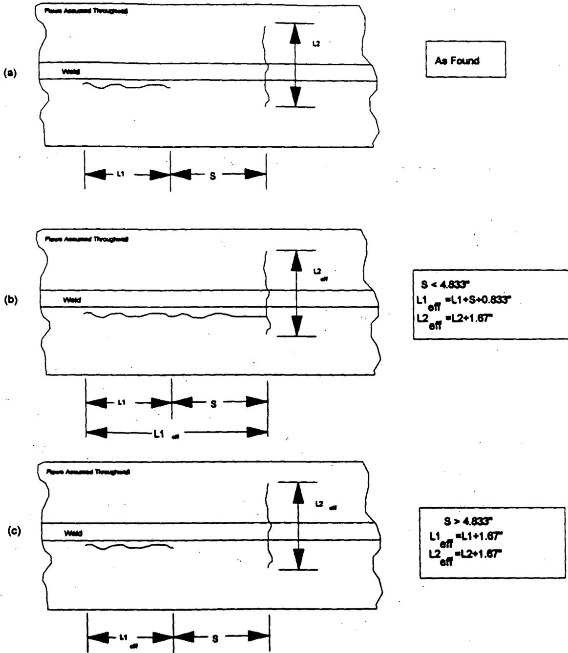
**Figure 2-3: Application of Proximity Procedure to Neighboring Axial and Circumferential Flaws**
