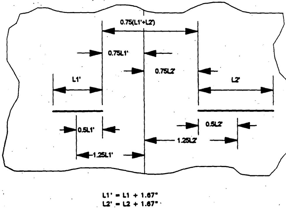
Figure 3-3: Schematic Illustrating Flaw Interaction
