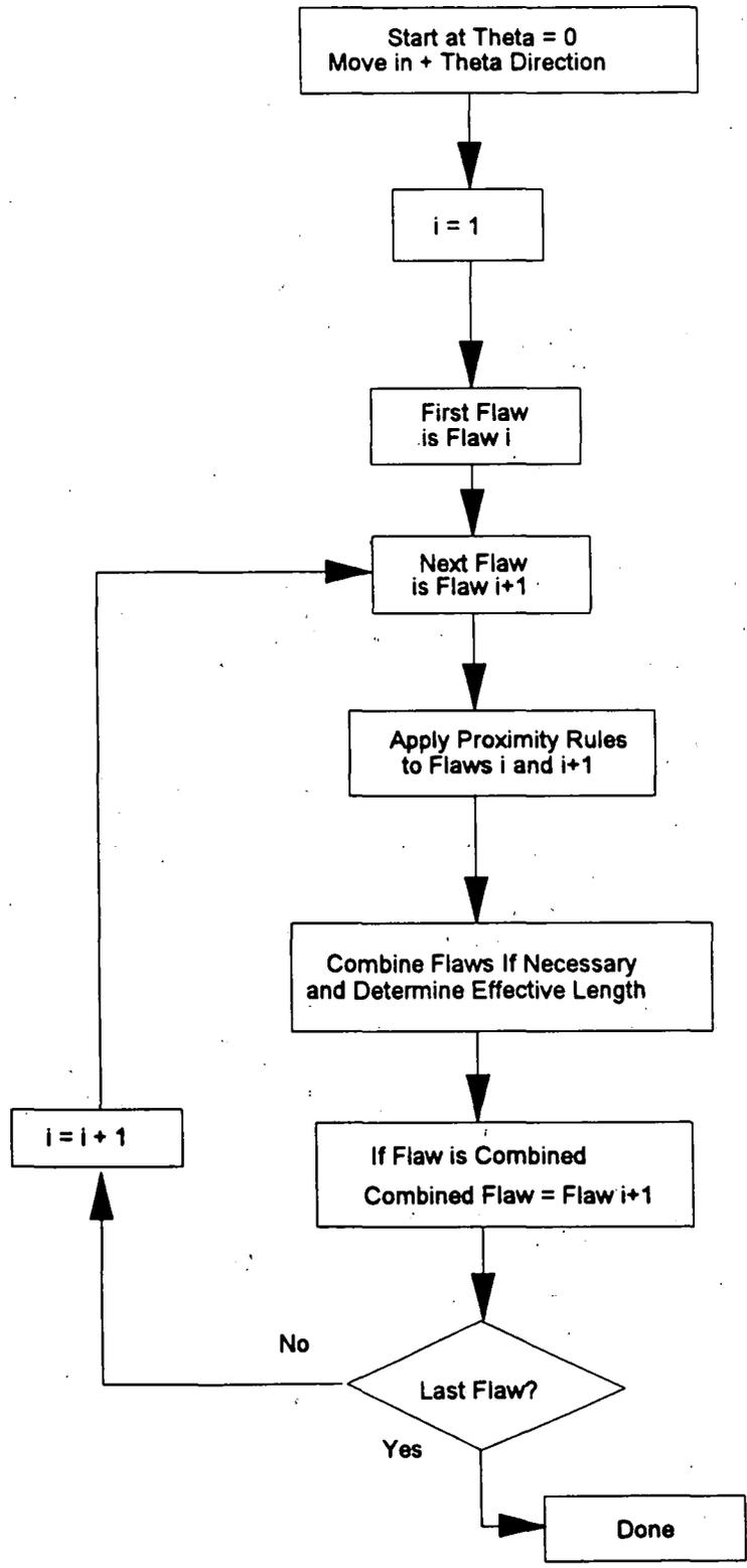
Figure 2-4: Process for Determining Effective Circumferential Flaw Length
