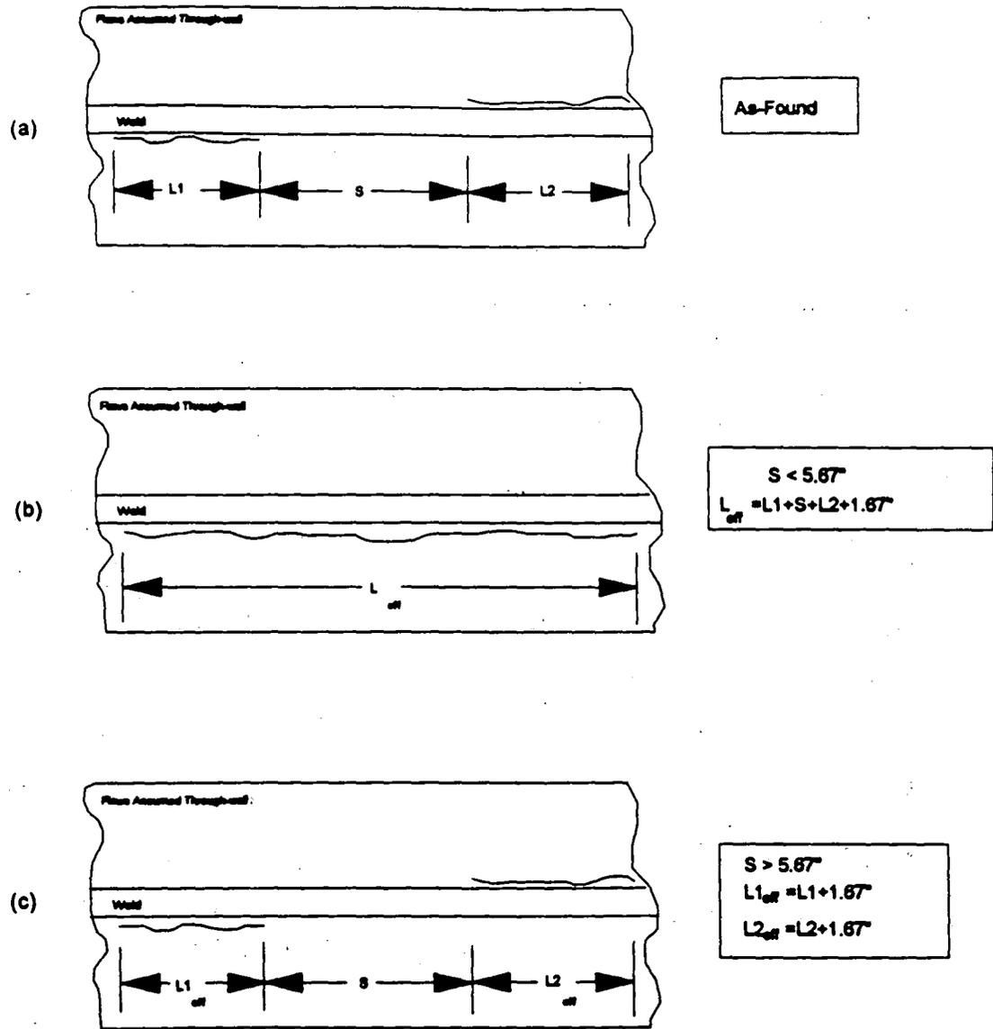
**Figure 2-2: Application of Proximity Procedure to Neighboring Circumferential Flaws**
