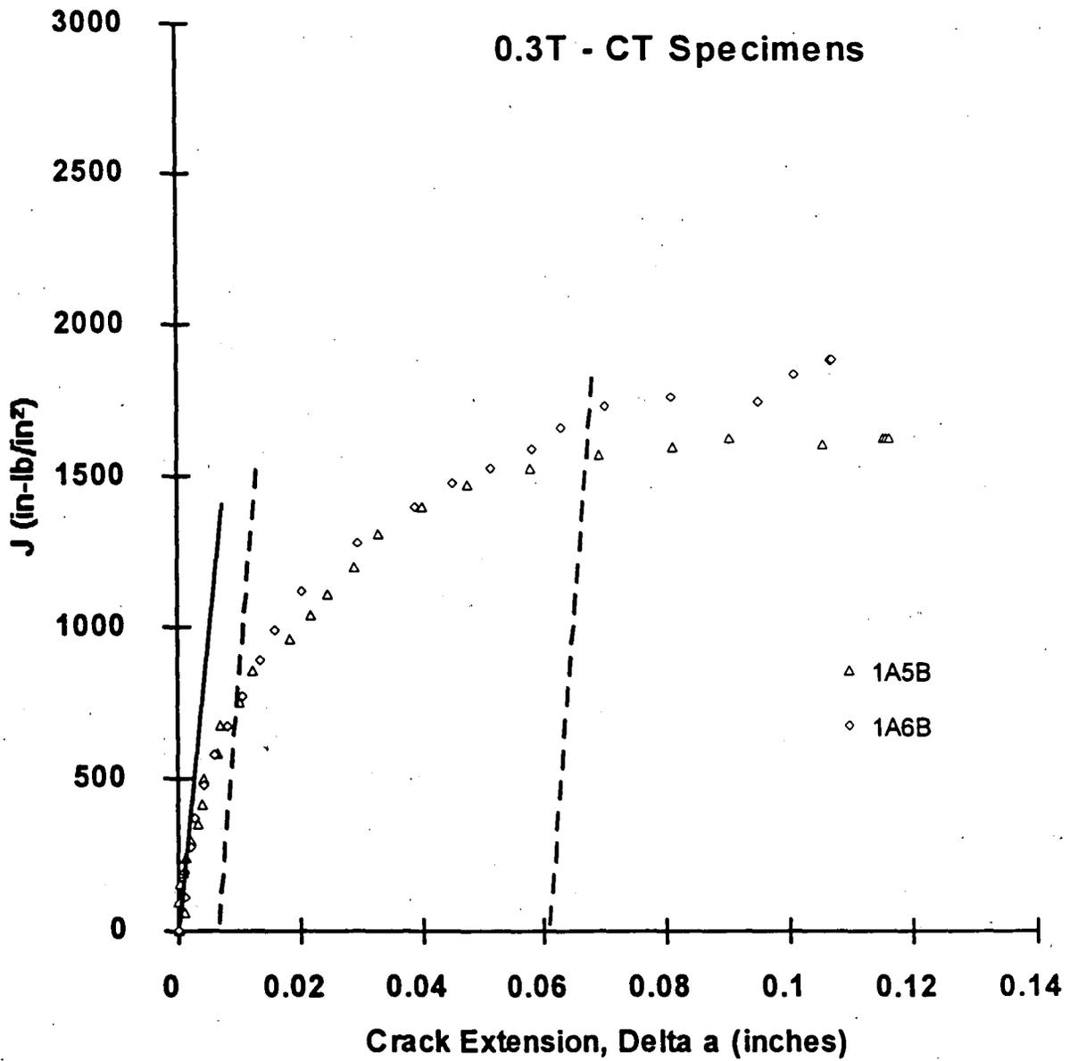
Figure 3-2: Comparison of J-R Curves Developed for Two Irradiated Stainless Steel Specimens
