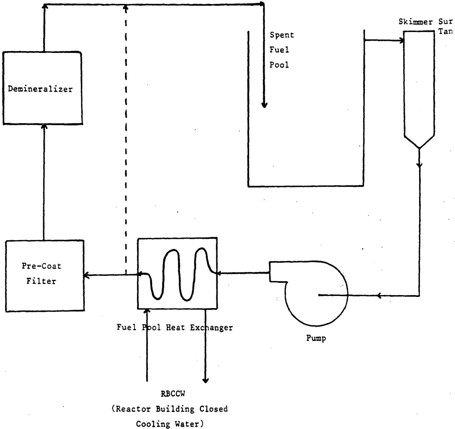
Figure 1: Simplified Flowpath for Fuel Pool Cooling and Cleanup System in a Normal Operation
