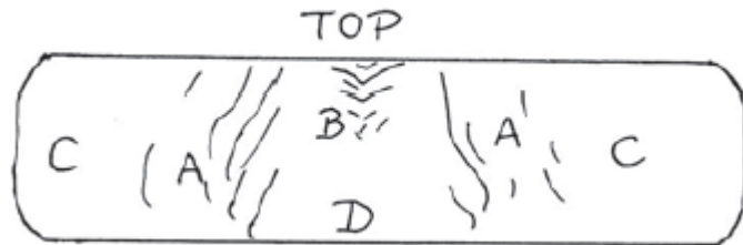
Upset disk, such as might be used for fabrication of a head
