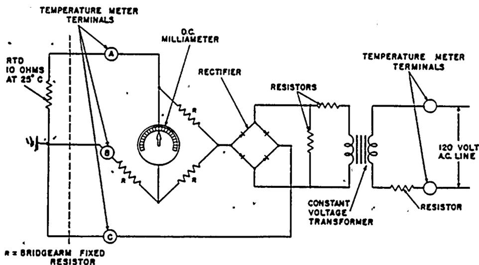
Fig. 1. RTD and temperature meter circuit (124C909)
