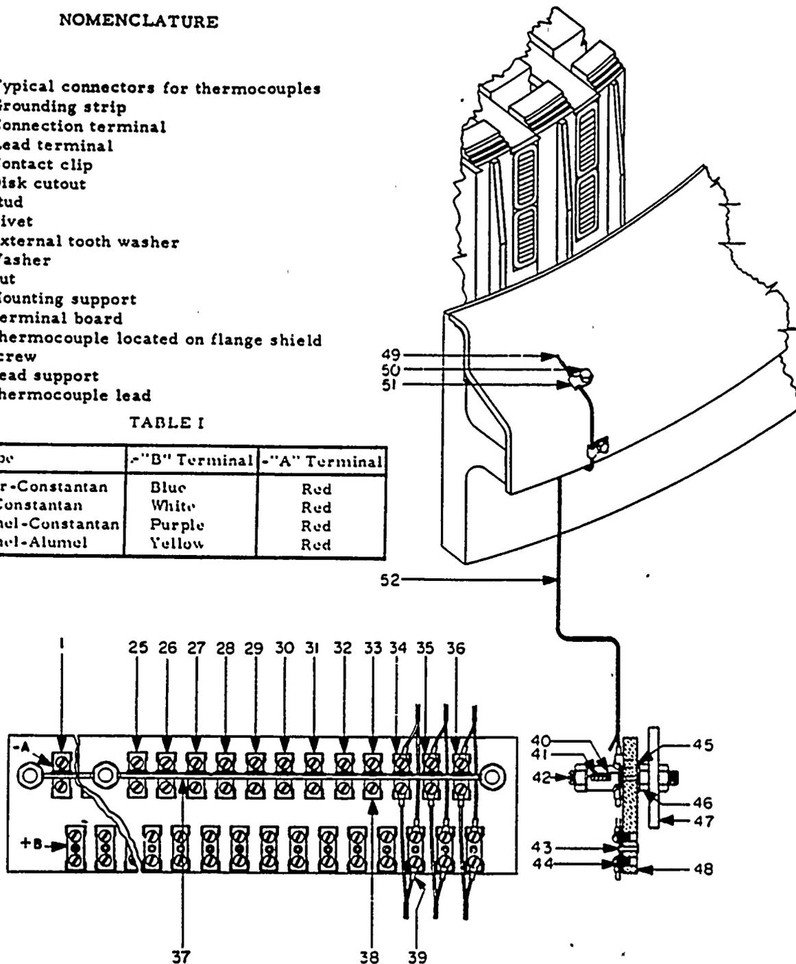
Fig. 1. Terminal board
