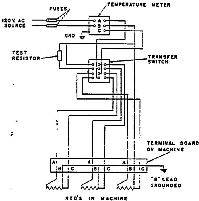
Fig. 3. RTD connections (124C908)
