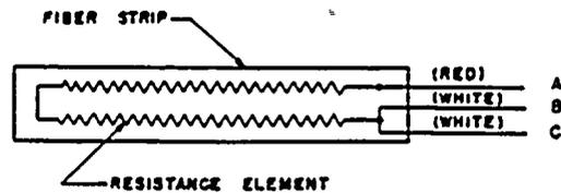
Fig. 4. RTD construction (762A122)
