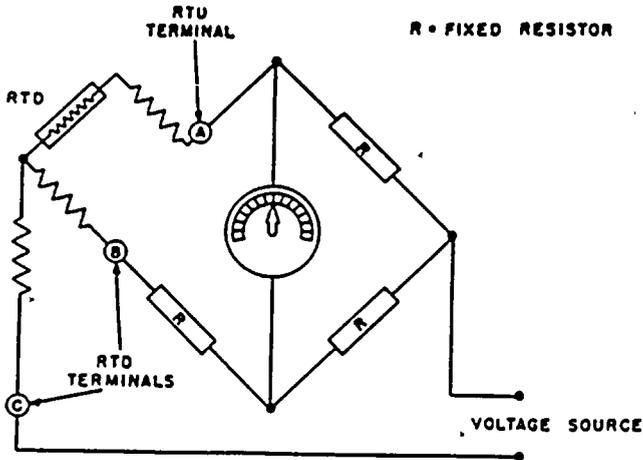
Fig. 2. RTD and Wheatstone Bridge circuit (762A123)
