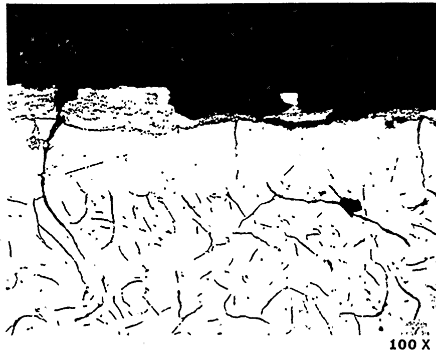
Figure B-53. Longitudinal cross-section of the non-thrust side of the B diesel 7L liner taken 16.5 inches from the bottom of the liner. Typical examples of the metal deposited from the piston and rings on the Cr plating.
