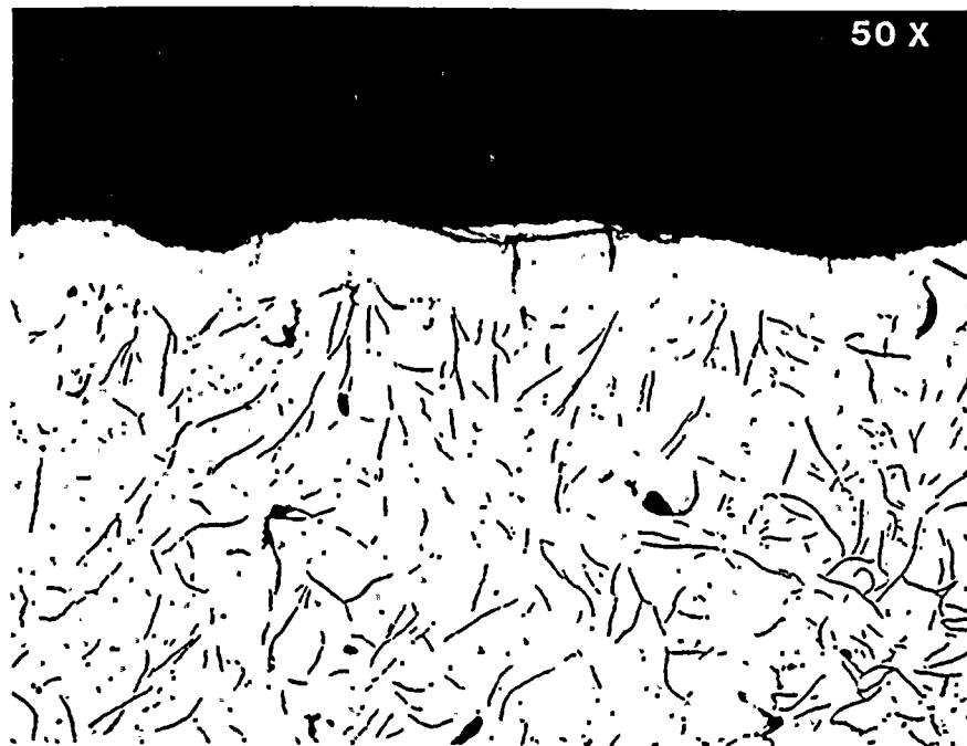
Figure B-30. Transverse cross-section (labeled area 'D') taken 7 1/2 inches from the bottom of the B diesel 7L liner showing depressions in the Cr plating surface, cracking of the base metal casting and deposited metal.
