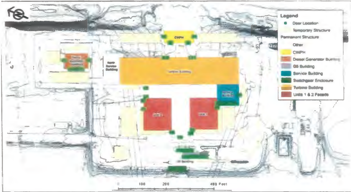
Figure 3.2-1. Permanent and Temporary Structures of the Point Beach Site, TS1 and TS2 are the temporary structures referenced in the Scenario A section. Source: FHRR Figure 4.5
