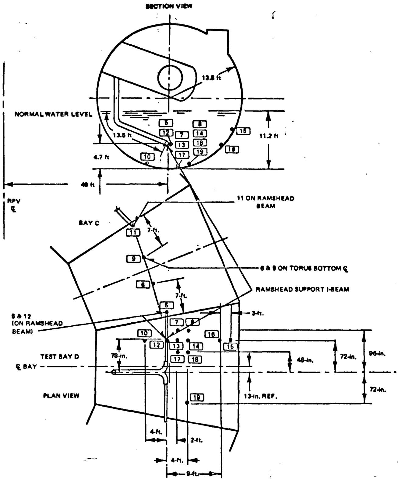
FIGURE 1) - Location of Pressure Transducers P5 through P19 in Torus Pool
