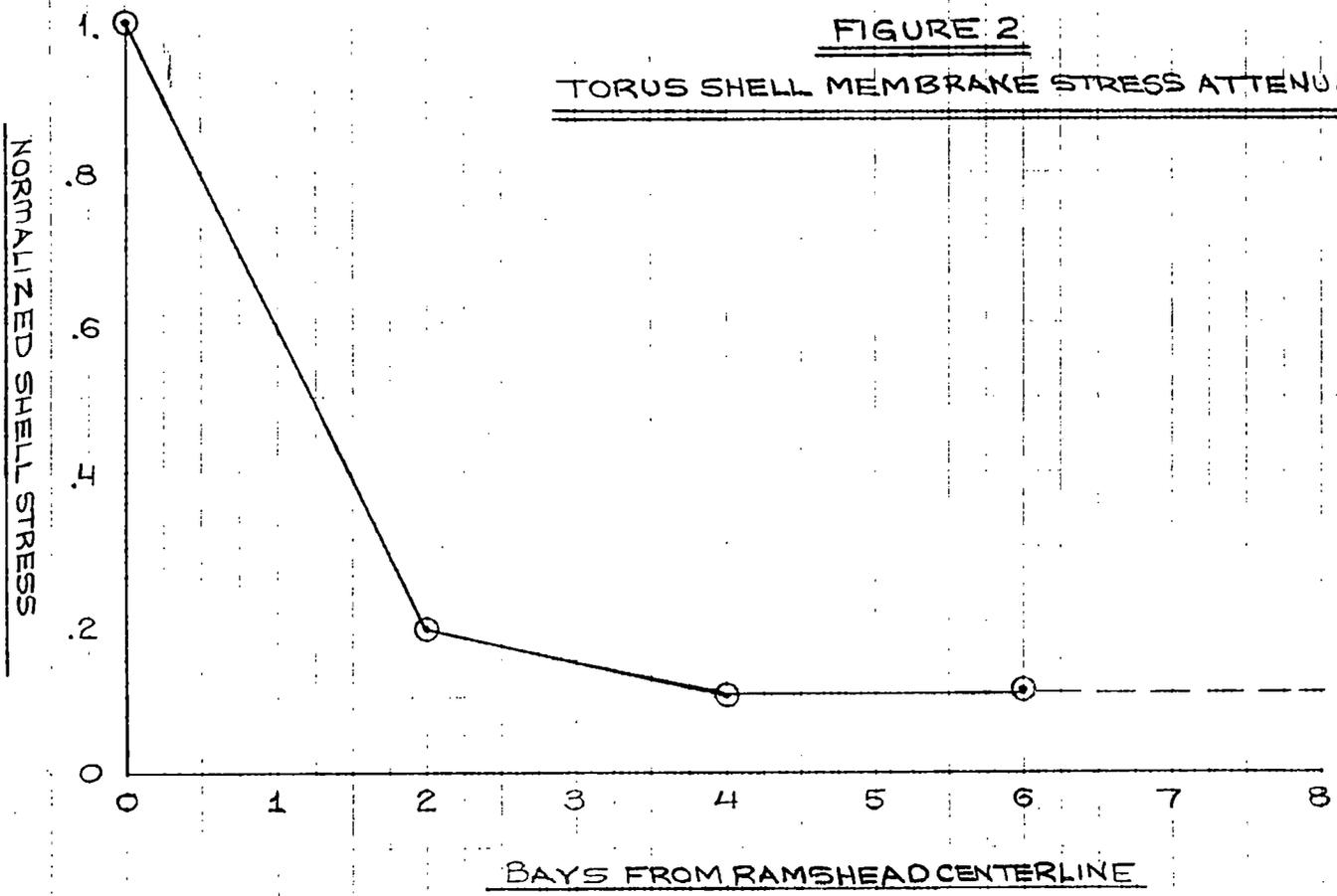
to comparative multiplier factors derived from the shell stresses recorded during multiple valve actuation tests. The data, method, and results of this comparison are shown in Figure 3. The conclusion drawn from this comparison was that there was good correlation between the multiple valve discharge strain gage data and the pressure based attenuation curve. The small differences in the results were attributed to the fact that the gages measured both the membrane and shell bending stresses.
