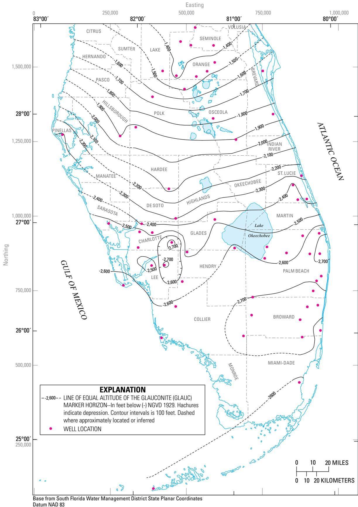
Figure 12. Altitude of the glauconite marker horizon.
