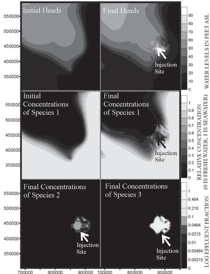
**Figure 3: Map view of the MFA showing initial heads and concentrations, and final heads and concentrations of species 1, 2, and 3 after 148 years of injection. Coordinates are in feet, State Plane 83.**
