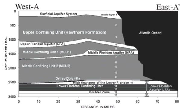
**Figure 1: Cross section showing hydrogeologic units along the eastern margin of the Florida Platform in southeastern Florida (Reese and Richardson, 2008; McNeill, 2002), geologic units and layering scheme used for numerical modeling. Location shown in Figure 2.**
