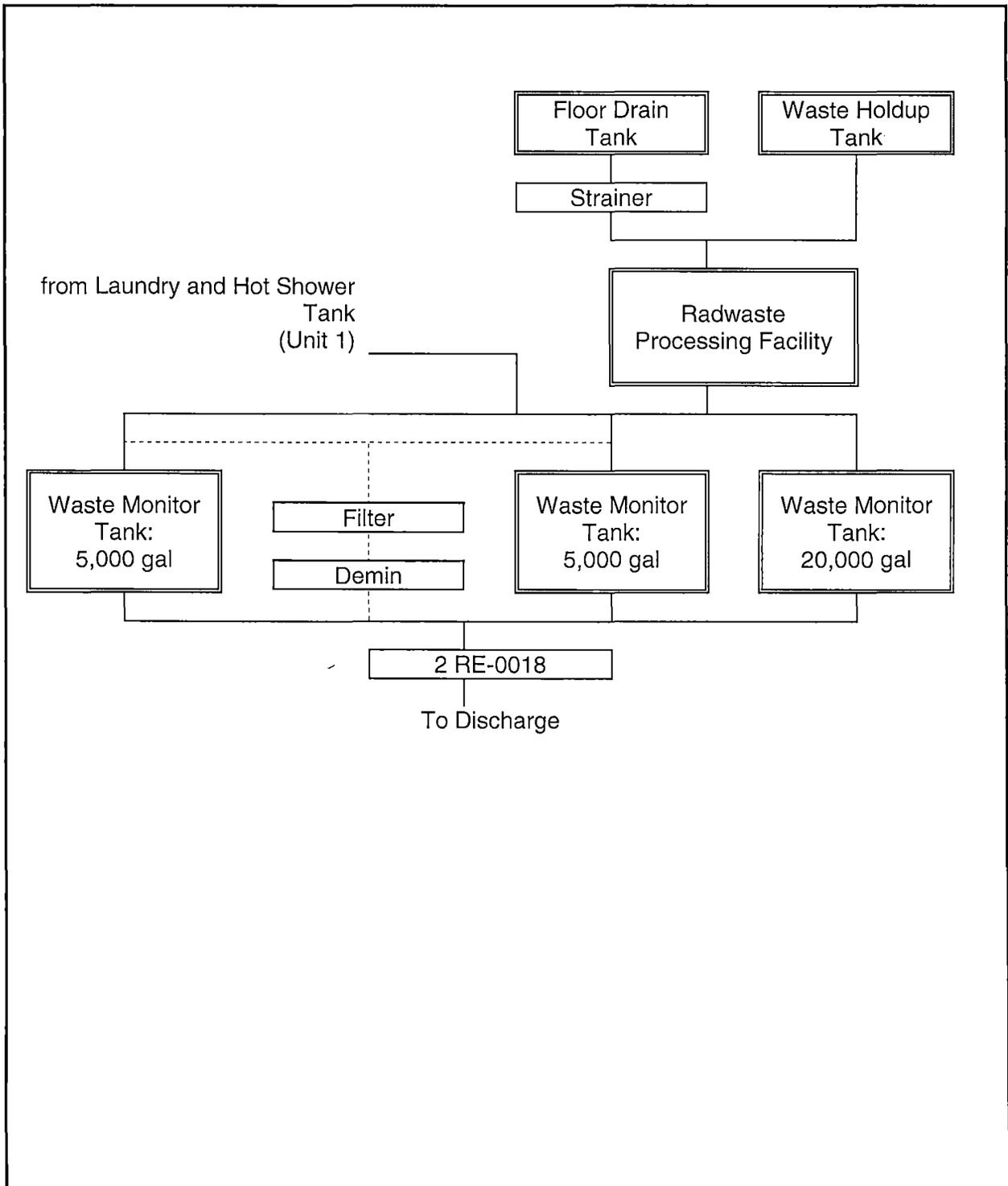
Figure 2-2. Unit 2 Liquid Radwaste Treatment System
