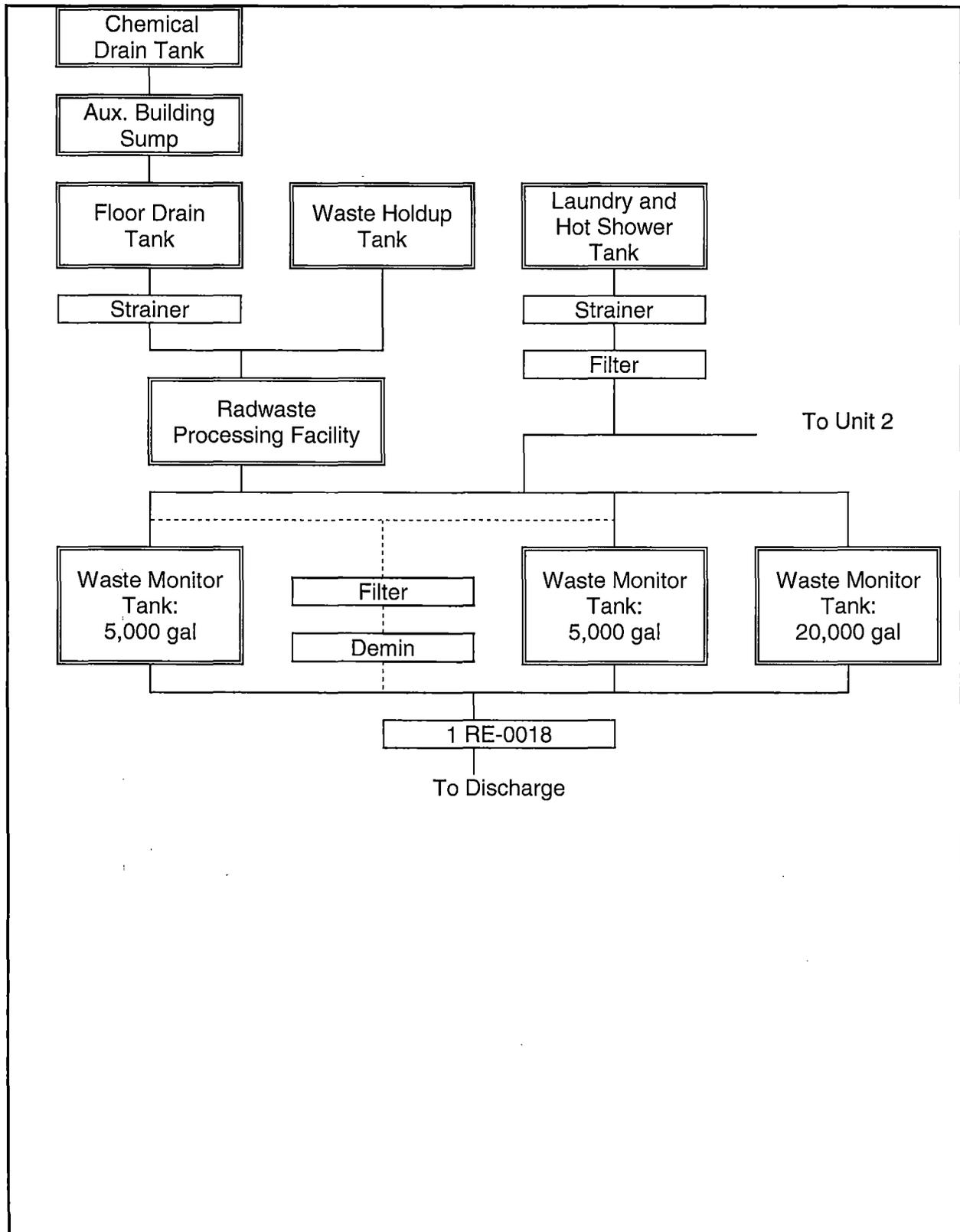
Figure 2-1. Unit 1 Liquid Radwaste Treatment System
