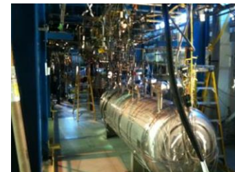
Mechanisms Engineering Test Loop (METL) facility at ANL – multiple test vessels for component testing in prototypic sodium conditions
