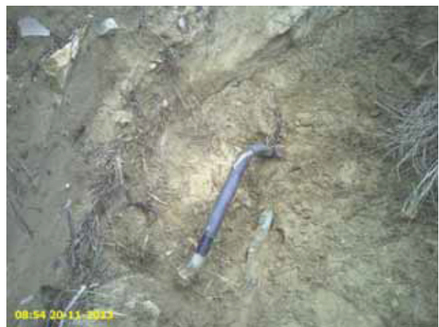
1-inch Plastic Coated Conduit Pipe, 3 ft long Reference Point 50 (11/20/13)
