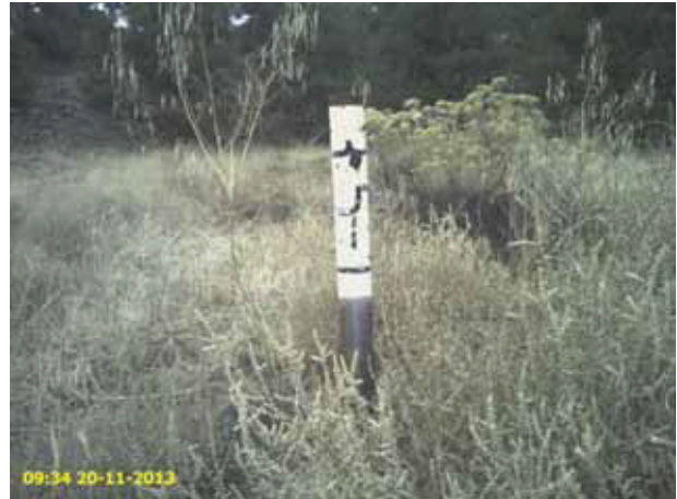
3-inch Metal Pipe (3 ft exposed) Reference Point 69 (11/20/13)
