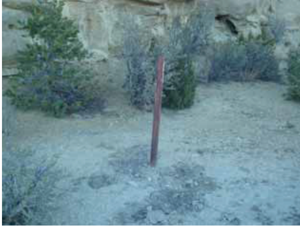
2.5-inch Steel Pipe (3.5 ft stickup) Reference Point 22 (11/11/13)
