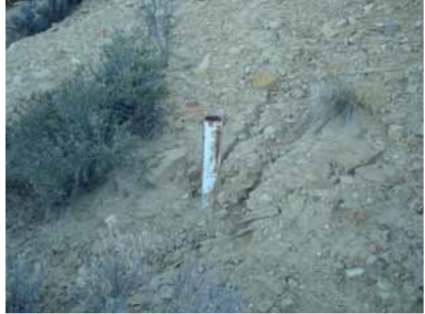
3.5-inch Steel Pipe (18 inch stickup) Reference Point 29 (11/11/13)
