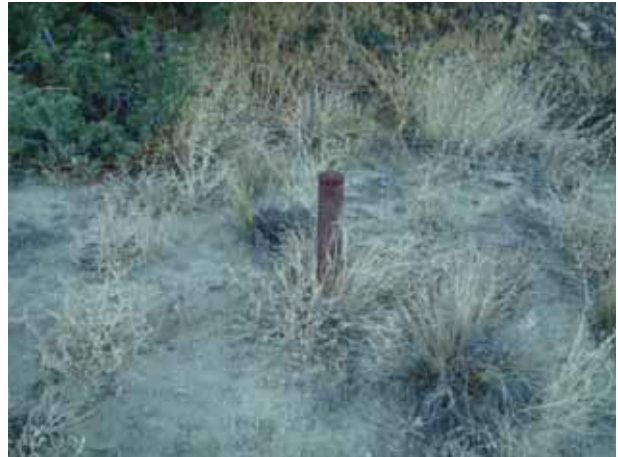
3.5-inch Metal Pipe (18 inch stickup) Reference Point 31 (11/11/13)
