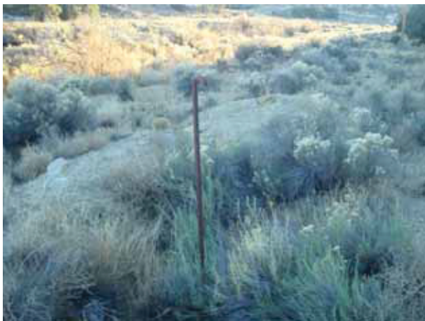
1-inch Steel Pipe (6 ft stickup) Reference Point 26 (11/11/13)
