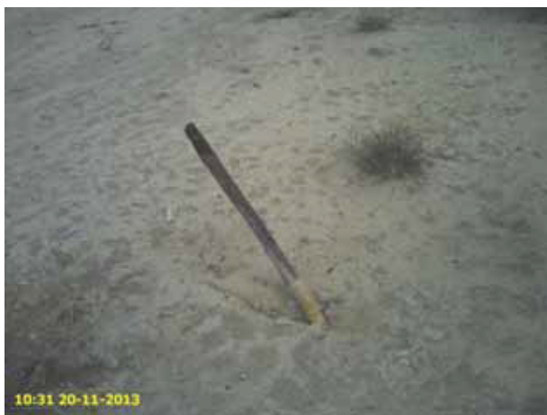
1.5-inch Metal Pipe (2 ft exposed) Reference Point 102 (11/20/13)
