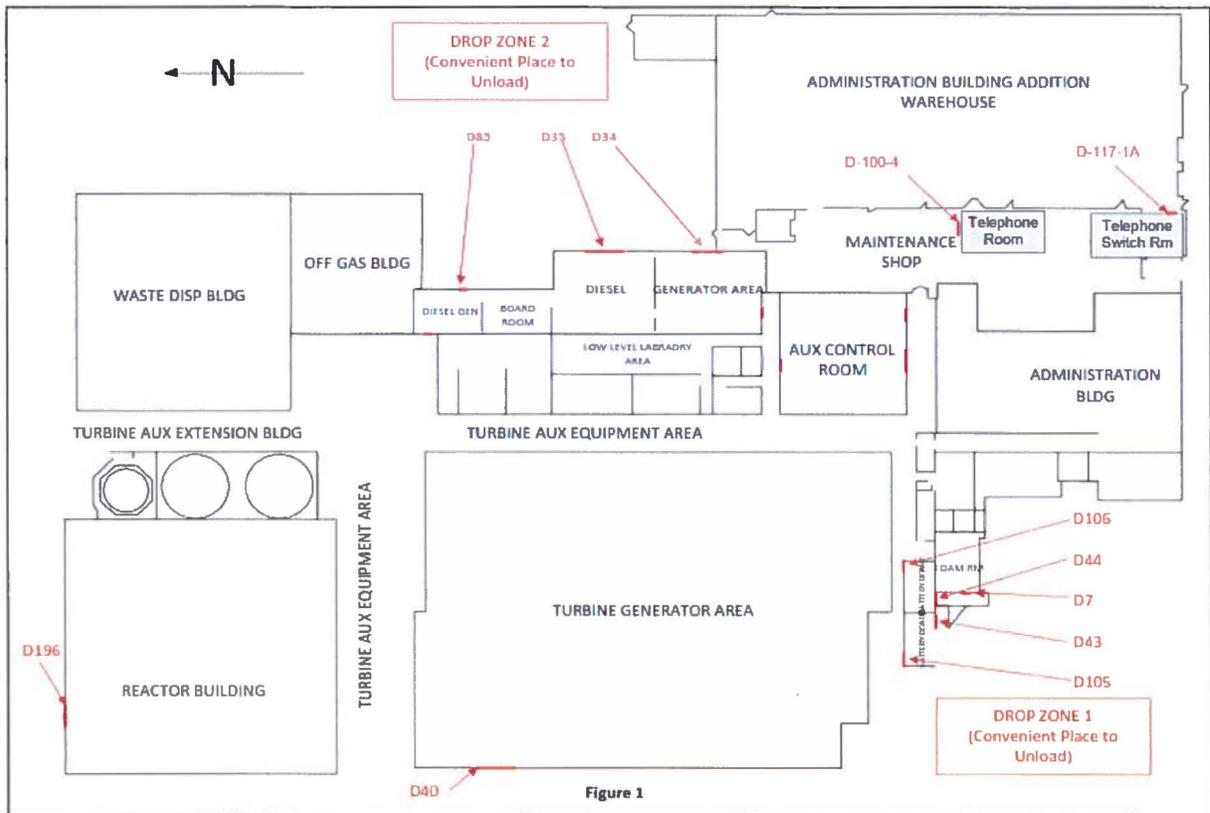
**Figure 7-2 – Location of Temporary Flood Protection Barriers in Unit 1**
