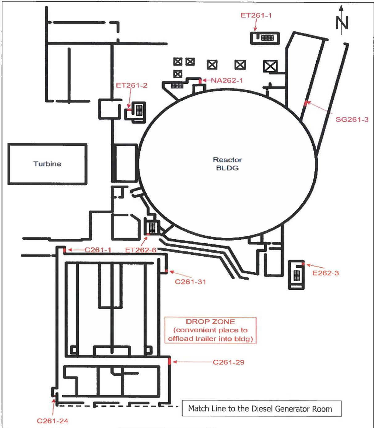
**Figure 7-4 - Location of Temporary Flood Protection Barriers in Unit 2**
