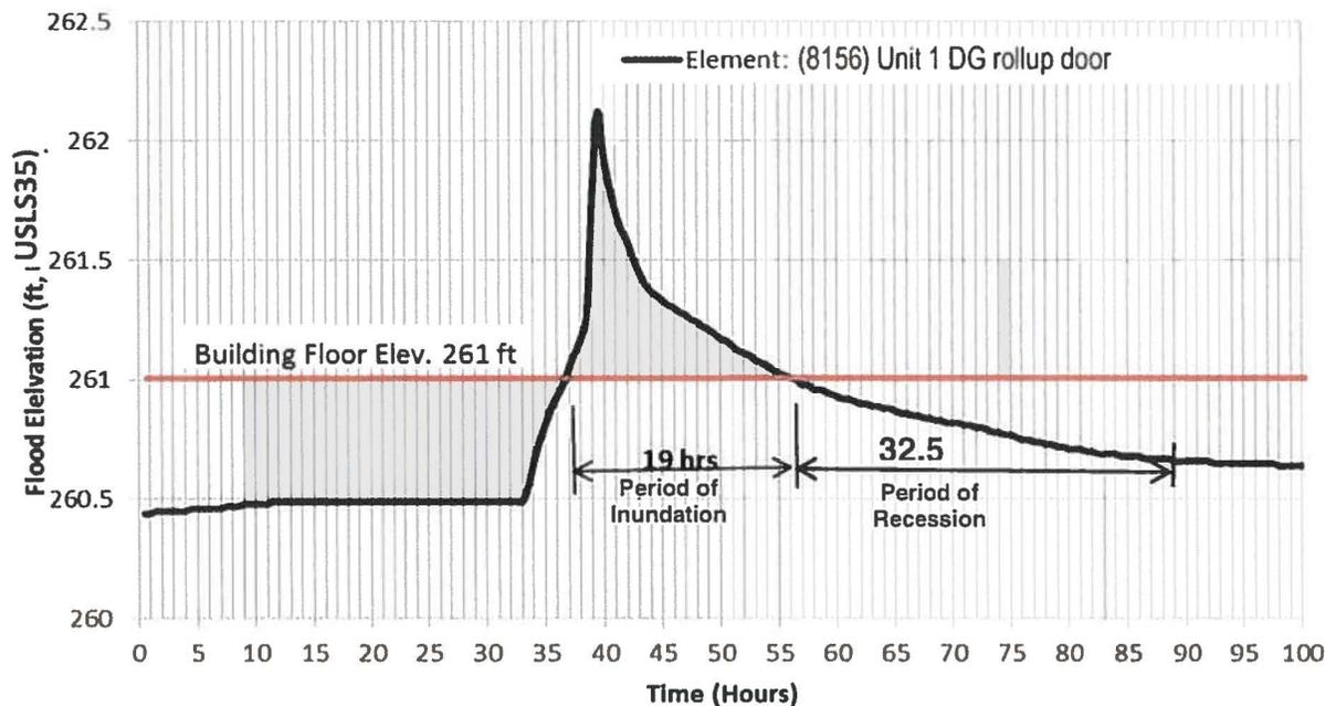
Figure 7-1 - 72-Hour LIP Water Surface Time Series Plot for Unit 1
