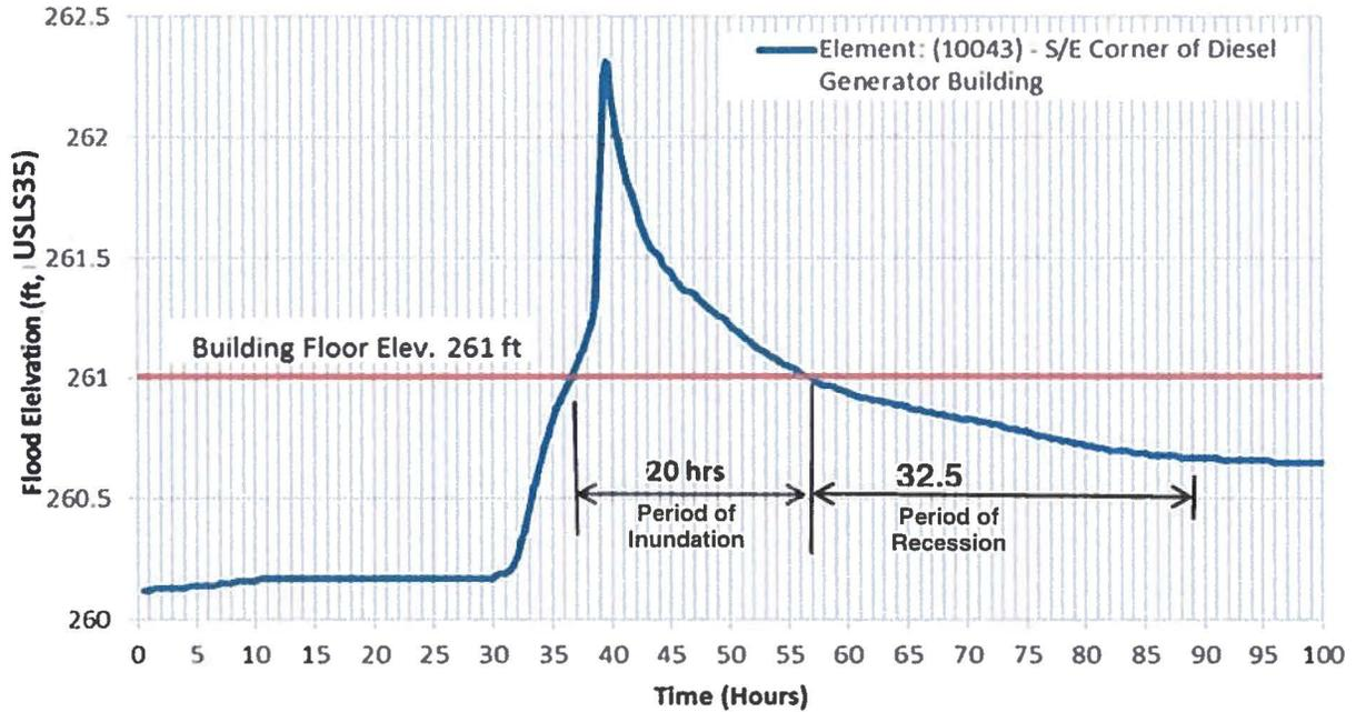
**Figure 7-3 - 72-Hour LIP Water Surface Time Series Plot for Unit 2**
