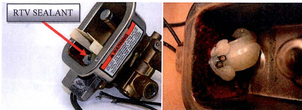
(NOTE: COIL LEAD WIRES WERE CUT TO REMOVE COIL)
