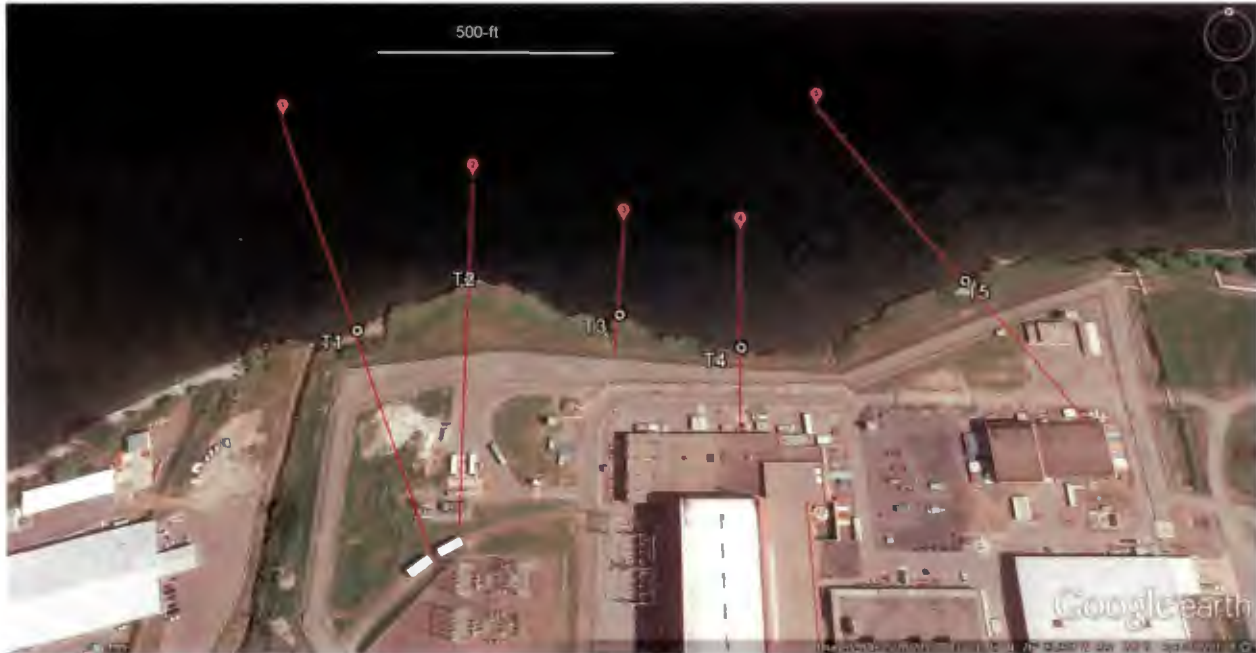
Figure 3.5-1. Wind-wave transects 1-5 and SWAN output locations (T1-T5) (adapted from FHRR unnumbered figure and FHRR Figure 3-44; locations are approximate); licensee determined that maximum combined flood hazard elevation location T5. (Base figure from Google Earth (Google Earth, n.d.))
