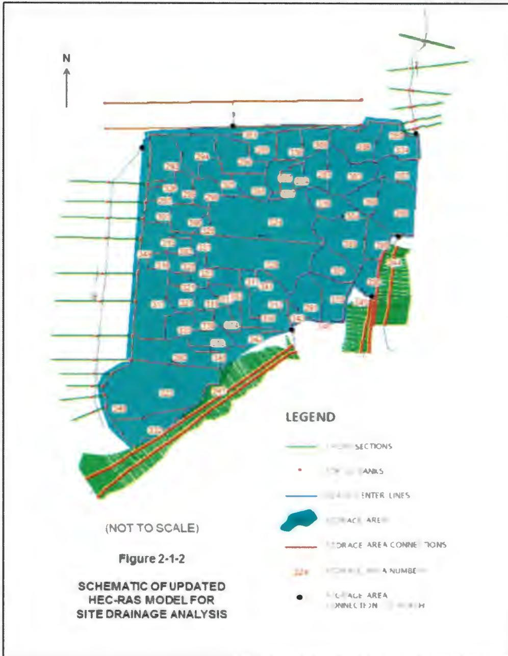
**Figure 3.2-2: Schematic of Updated HEC-RAS Model for Site Drainage and LIP Analysis
