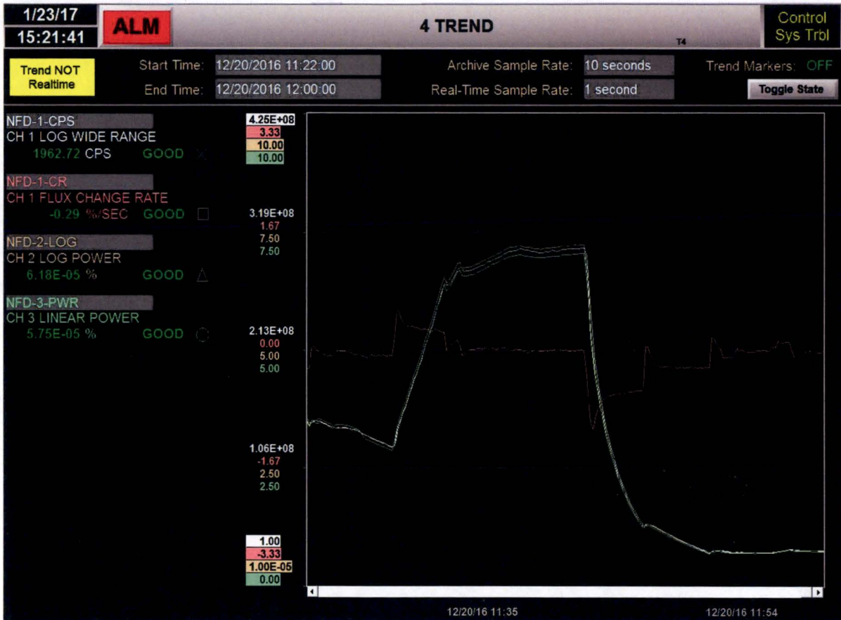
Figure 7-8: Example Trend Showing Channels 1-3 Level and Channel 1 Change Rate for an example run
