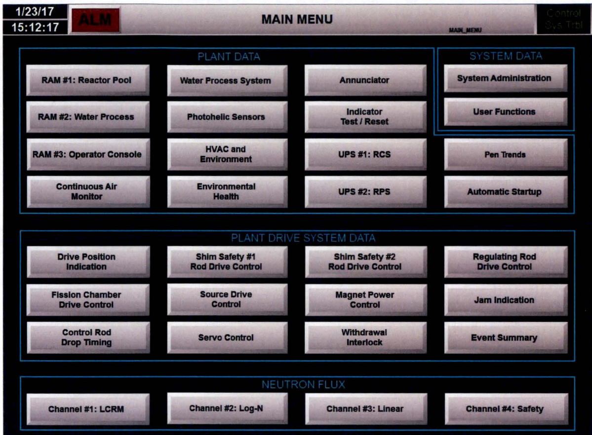
Figure 7-6: Summary Screen of Reactor Control System
