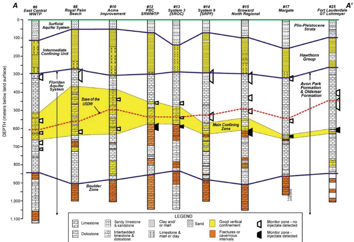
**Fig. 2** Hydrogeologic cross section through southern Palm Beach County and North Broward County Florida showing locations of high transmissivity (fractured strata), confining strata, and monitoring zones. The base of the deepest USDW is marked
