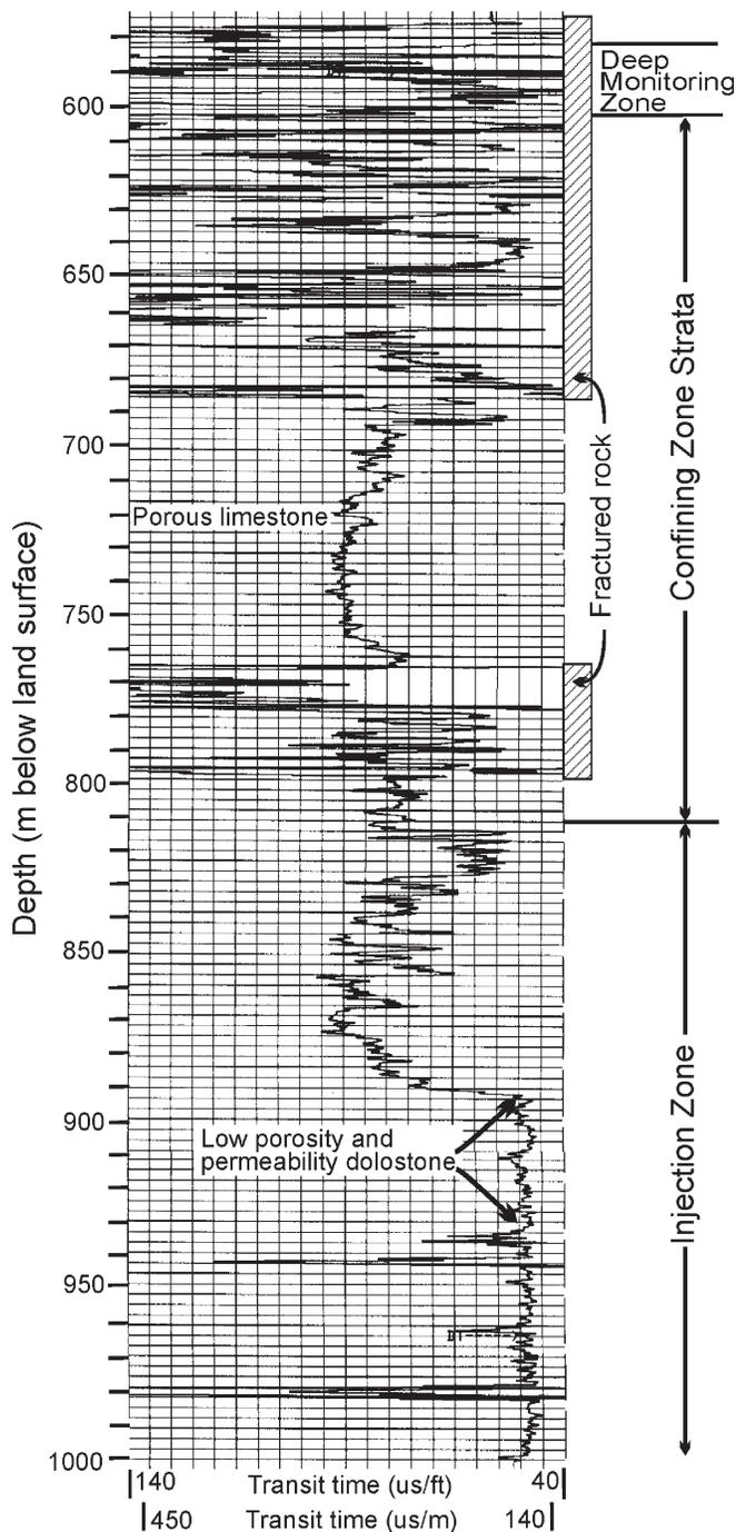
**Fig. 4** Sonic log from the Palm Beach County SRWWTP injection well system (IW-1), which experienced rapid vertical migration of injected wastewater into a deep monitoring zone. Fractured strata are characterized by very long transit times. Strata with low hydraulic conductivities, as indicated by short transit times, are not present between the injection zone and lower monitoring zone
