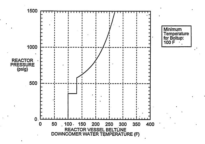
(reactor vessel beltline downcomer water temperature is measured at recirculation loop suction) (instrument uncertainties have been included in this figure)
