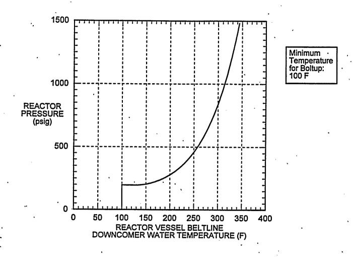
(reactor vessel beltline downcomer water temperature is measured at recirculation loop suction) (instrument uncertainties have been included in this figure)
