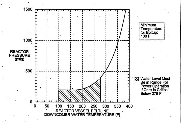
(reactor vessel beltline downcomer water temperature is measured at recirculation loop suction) (instrument uncertainties have been included in this figure)
