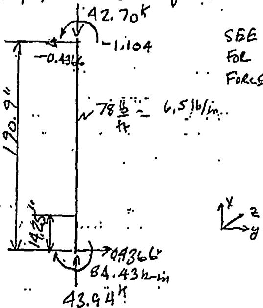
$$\text{Axial } \Rightarrow 14.25'' = 43.94^k - (14.25'') \left( \frac{6.5 \text{ lb/in}}{1000} \right) = 43.85^k (\text{C})$$
