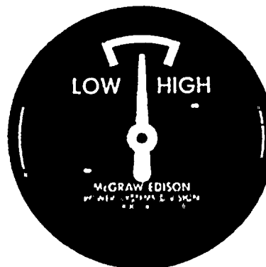
Figure 2. Magnetic oil-level gage showing normal oil level.
