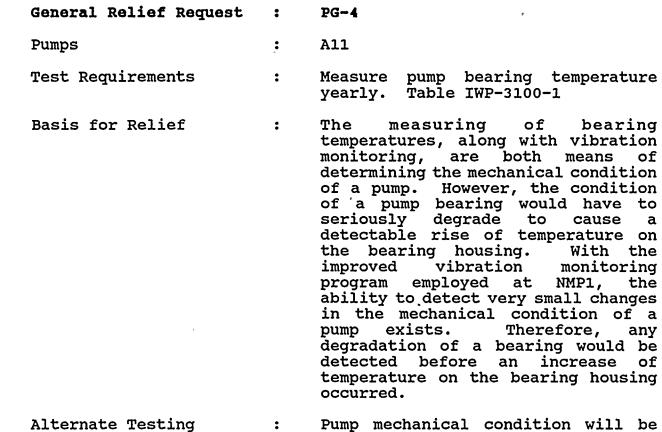
Alternate Testing : Pump mechanical condition will be determined by the enhanced vibration monitoring program. Bearing temperatures will not be measured.
