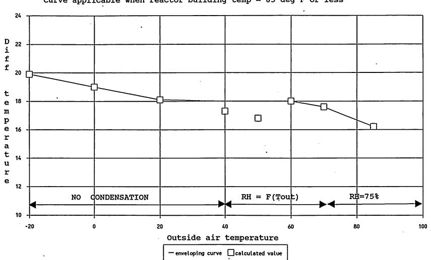
NMP2 Drawdown Analysis 1st refueling, 90 DAR Curve applicable when reactor building temp = 85 deg F or less
