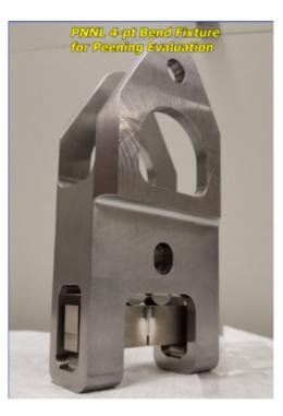
PNNL concept for crack arrest specimen by Dr. Mychailo Toloczko
