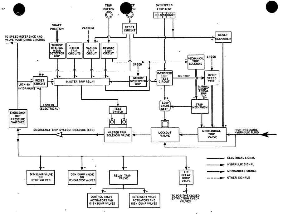
Fig. 1. Signal flow chart for emergency tripping system, EHC
