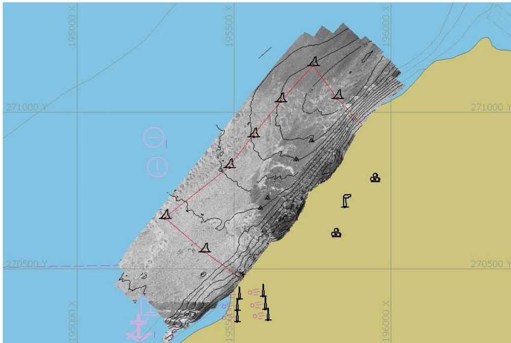
**Figure B-2. Sidescan imagery from the April 2010 survey performed by Substructure Inc. Gray color indicates the degree of acoustic backscatter from sediment on the river bed. Dark gray tones were considered to be areas of fine grained sediment while the light gray areas represented coarse grain deposits. Lines indicate water depth which decreases from upstream to downstream and near shore.**
