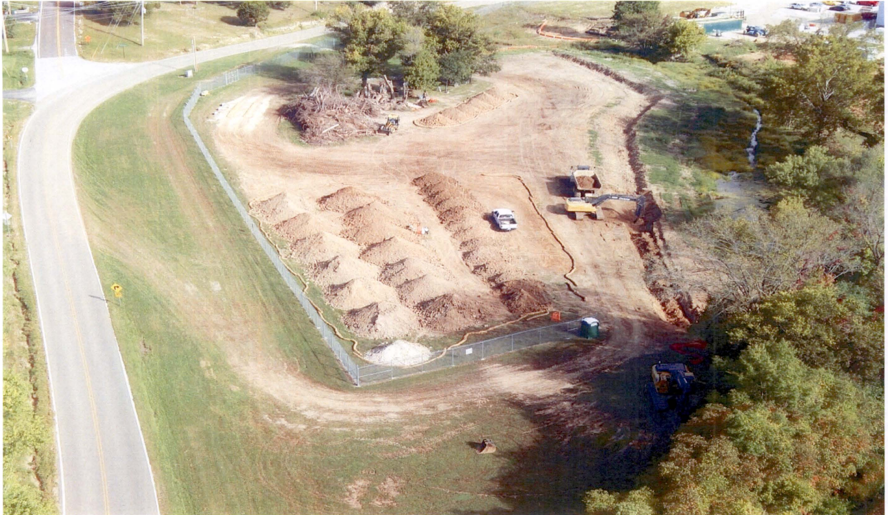
Figure 2-61 Installation of the Site Pond Diversion Ditch Which Was Constructed To Divert Water From The Site Spring Around And Downstream Of The Site Pond (Looking N)
