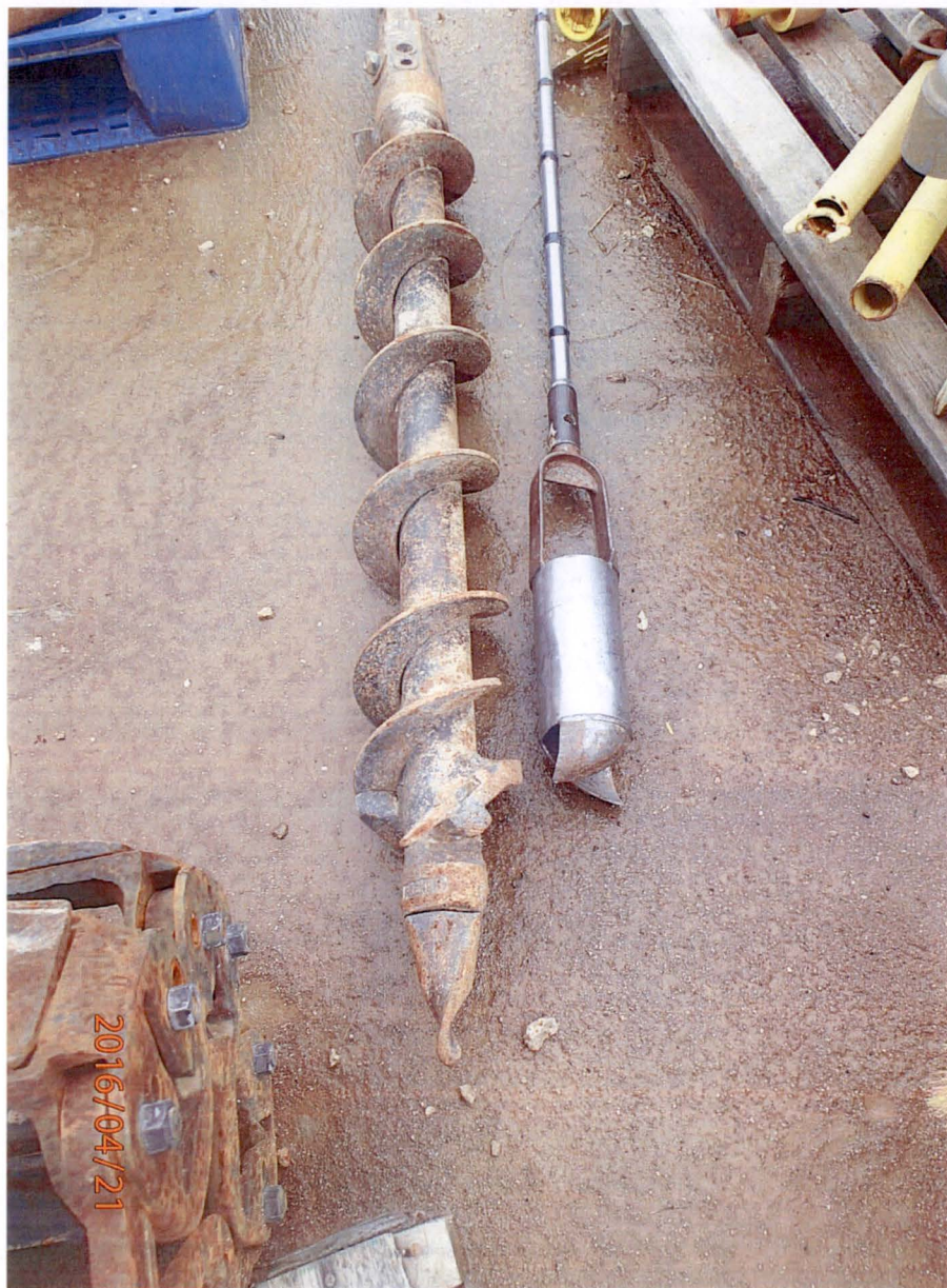
Figure 2-18a Example of Auger Types Used to Perform NCS Borings
