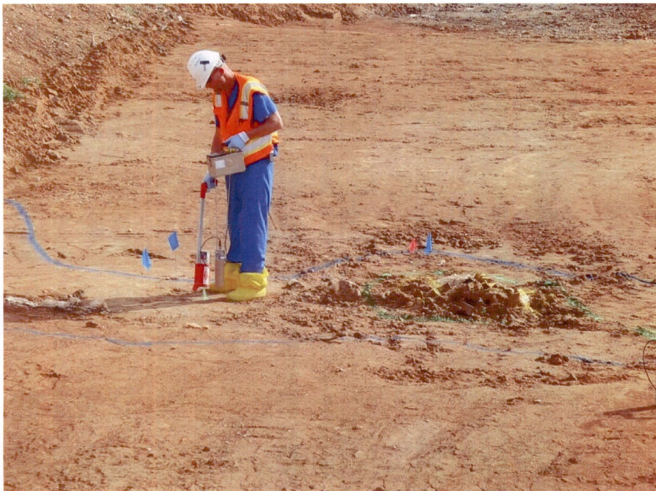
Figures 2-4 Example of Worker Conducting a Gamma Walkover Survey (GWS) in the Burial Pit Area with a NaI 2 x 2 Detector
