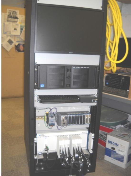
**Figure 1-4 High-Speed Data Logger**
