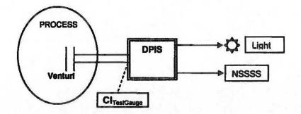
Note: Calibration tools are shown with dotted lines since these instruments are connected only during calibration. Only tools used for the calculating the system setpoints are shown. Calibration standards are not shown. The Light has no error.
